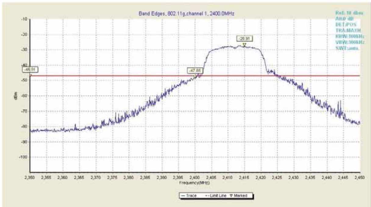
Fig27. Frequency Band Edges of 802.11g in channel 1,2412MHz
