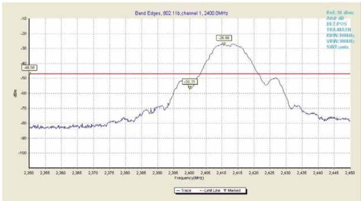
Fig25. Frequency Band Edges of 802.11b in channel 1,2412MHz
