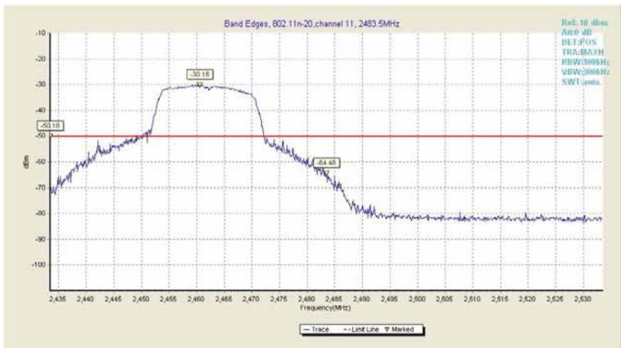
Fig30. Frequency Band Edges of 802.11n-20 in channel 11,2462MHz
