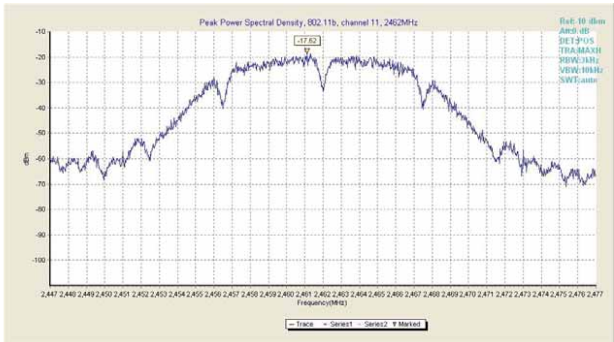
Fig.3 Peak power spectral density of 802.11b in channel 11,2462MHz
