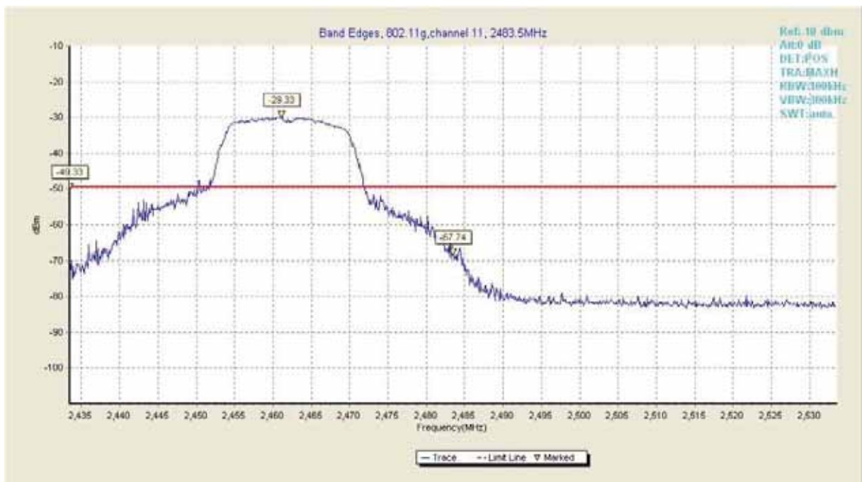
Fig28. Frequency Band Edges of 802.11g in channel 11,2462MHz
