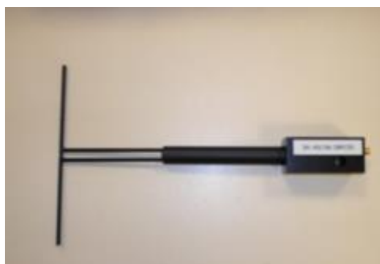
Figure 1 – Satimo COMOSAR Validation Dipole
