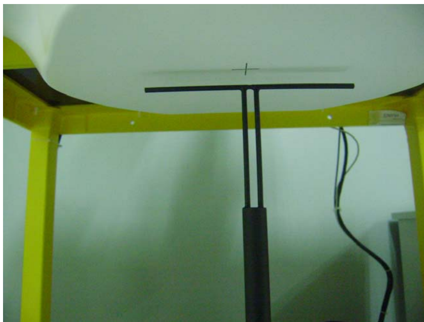
Fig 7.2 Setup Photo of Dipole Antenna
