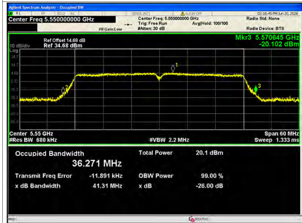
-26dB Bandwidth NVNT ac40 5550MHz Ant1
