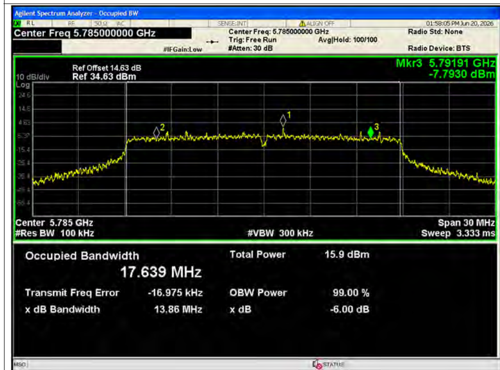
-6dB Bandwidth NVNT ac20 5785MHz Ant1
