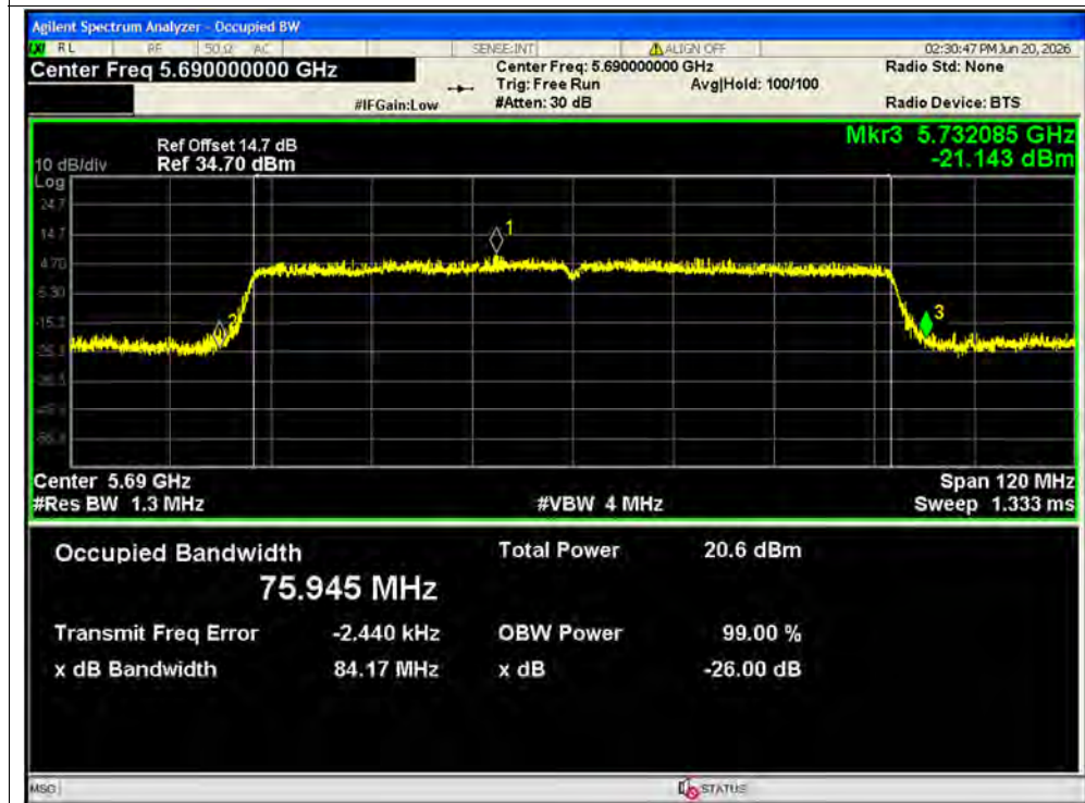
-26dB Bandwidth NVNT ac80 5690MHz Ant1
