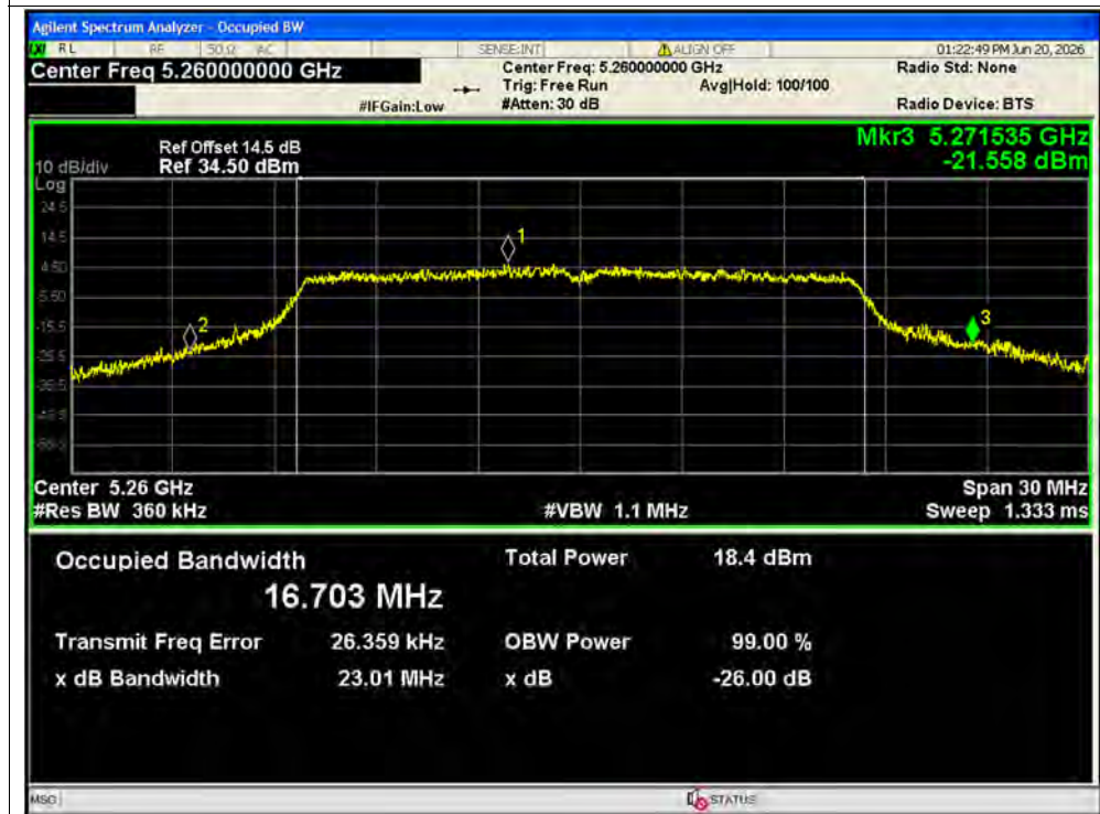
-26dB Bandwidth NVNT a 5260MHz Ant1
