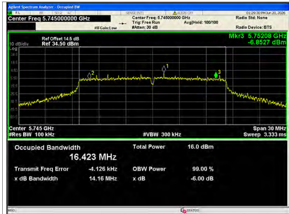
-6dB Bandwidth NVNT a 5745MHz Ant1
