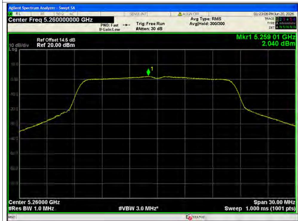
PSD NVNT a 5260MHz Ant1
