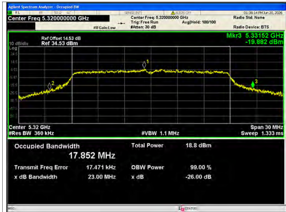
-26dB Bandwidth NVNT n20 5320MHz Ant1
