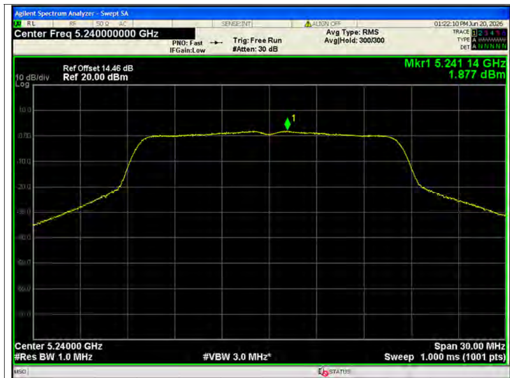
PSD NVNT a 5240MHz Ant1
