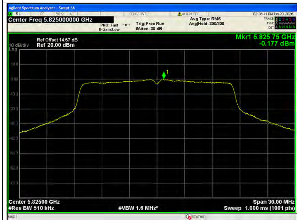
PSD NVNT a 5825MHz Ant1
