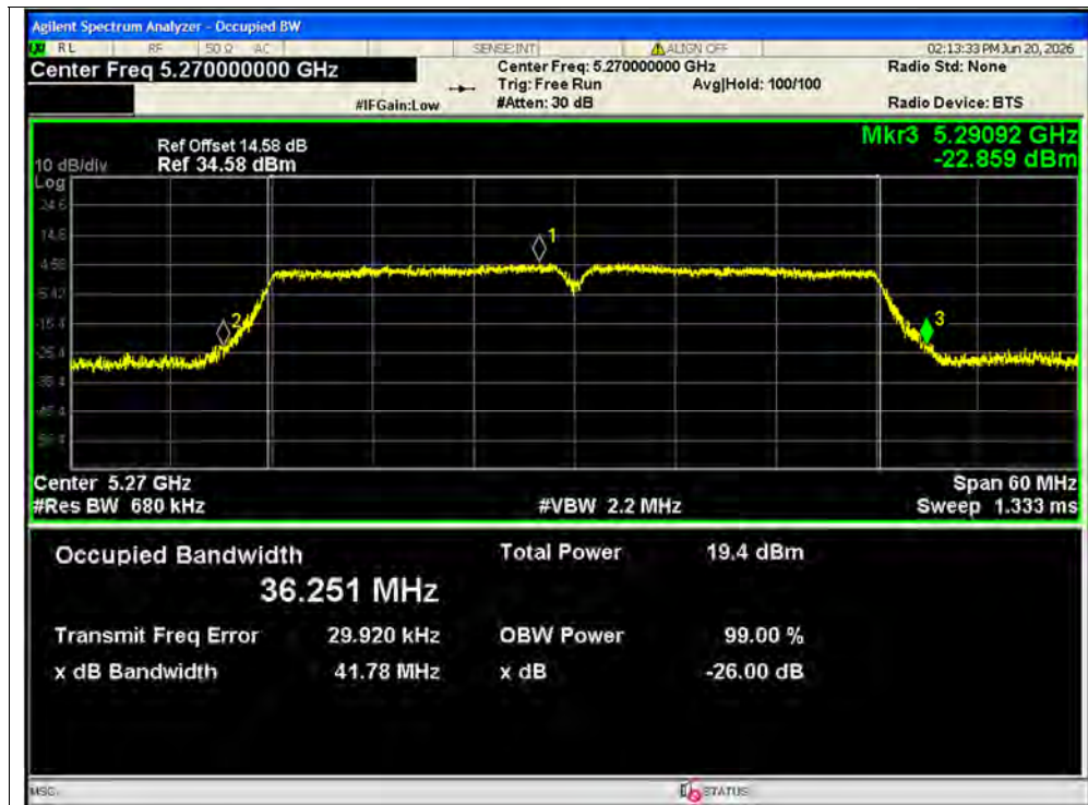
-26dB Bandwidth NVNT ac40 5270MHz Ant1
