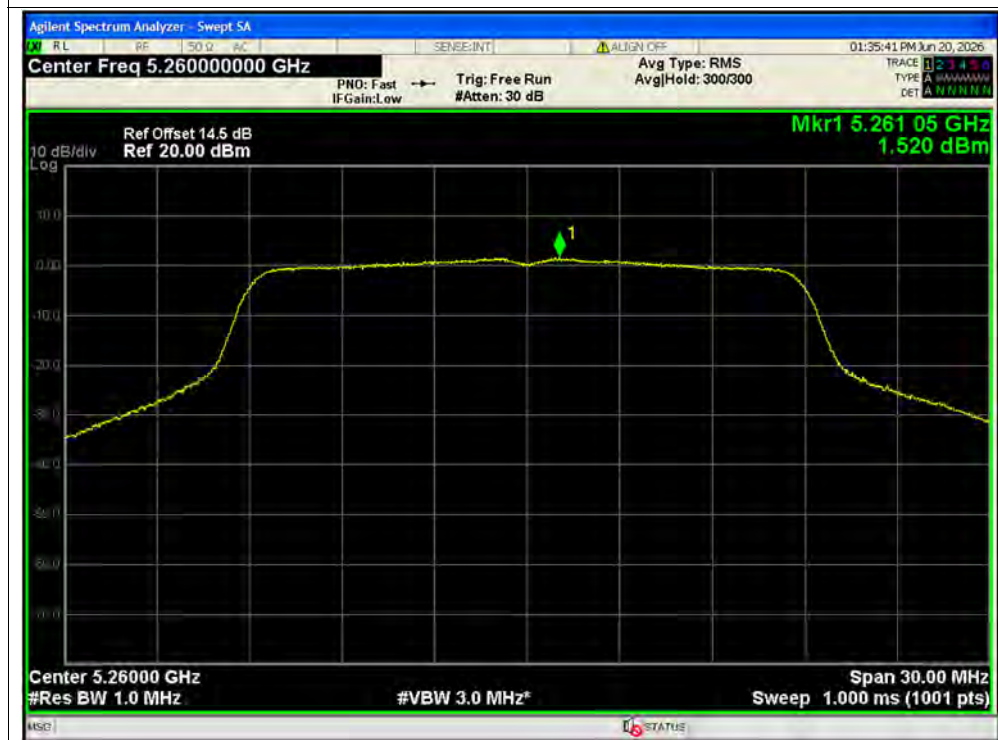
PSD NVNT n20 5260MHz Ant1
