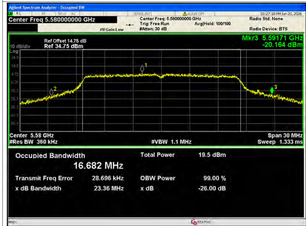
-26dB Bandwidth NVNT a 5580MHz Ant1
