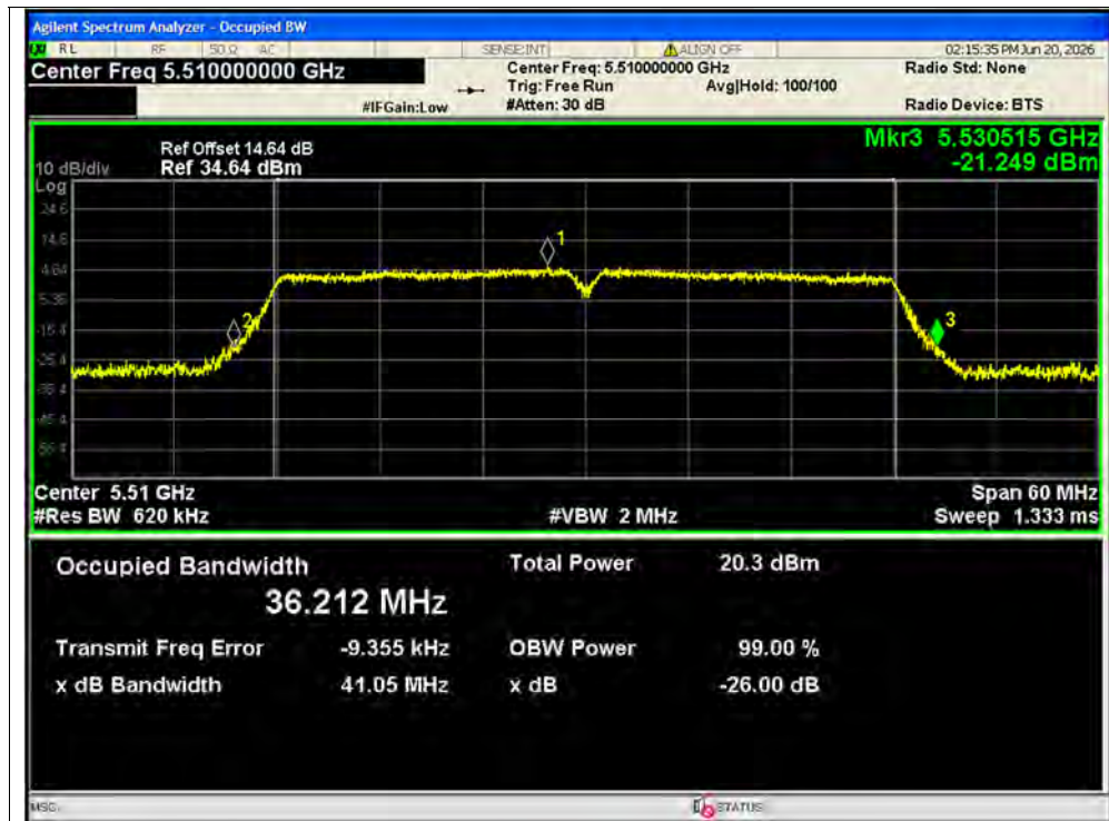
-26dB Bandwidth NVNT ac40 5510MHz Ant1
