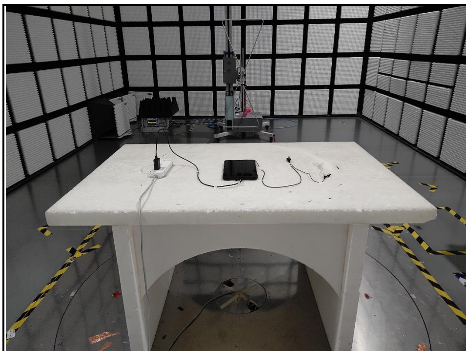
Fig. 2 Radiated emission setup photo(30MHz-1GHz)
