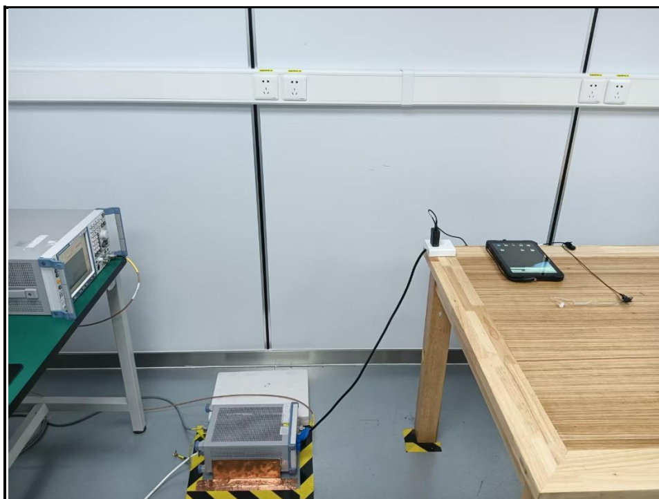
Fig. 3 Power line conducted emission setup photo
