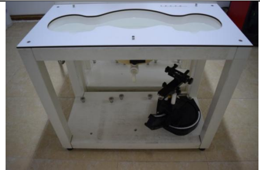
Fig. 6.6 Photo of SAM Phantom
