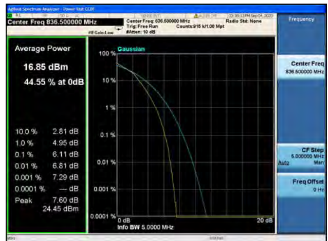
Band5 / 1.4MHz / High CH / 16QAM
