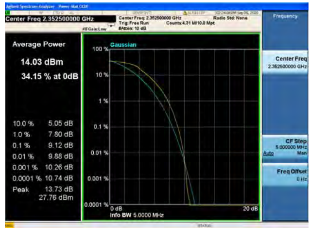
Band40/ Block B / 5MHz / Mid CH / 16QAM
