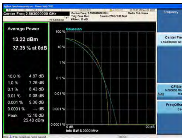
Band41 / 5MHz / High CH / 16QAM
