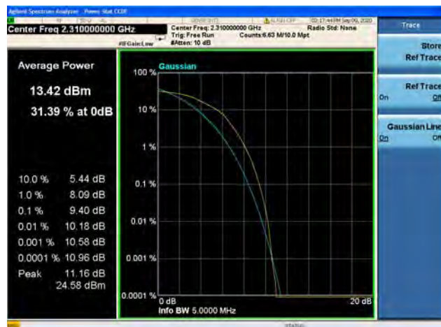
Band40/ Block A / 5MHz / High CH / QPSK
