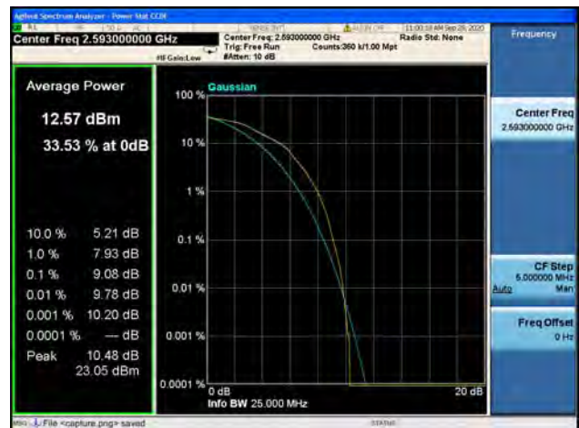
Band41 / 20MHz / High CH / 16QAM
