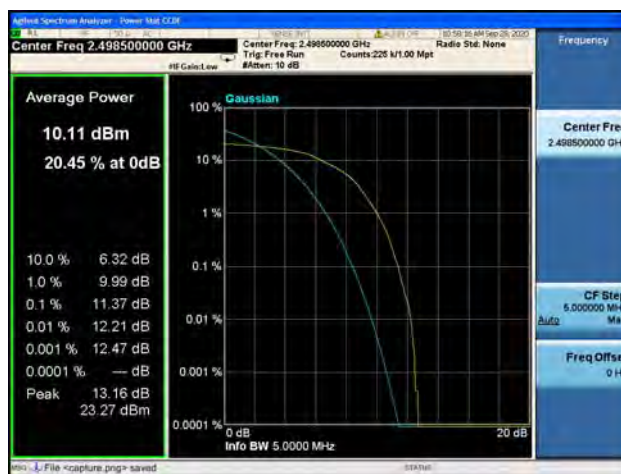
Band41 / 5MHz / Mid CH / 16QAM
