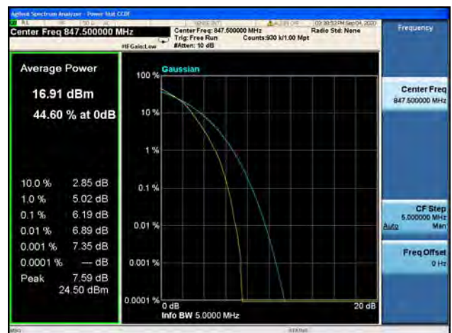
Band5 / 3MHz / High CH / 16QAM
