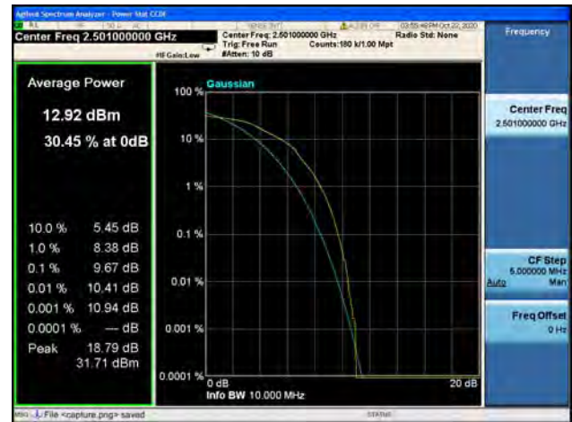
Band41 / 10MHz / Mid CH / 16QAM
