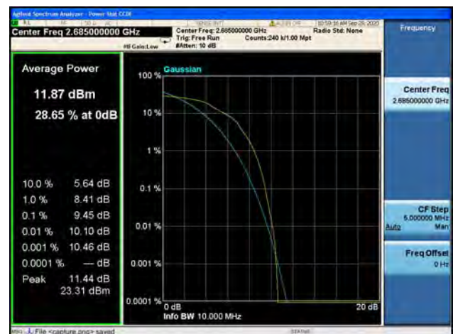
Band41 / 10MHz / High CH / 16QAM
