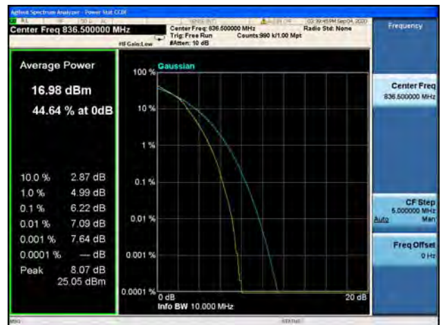
Band5 / 10MHz / High CH / 16QAM
