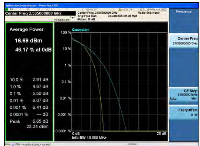
Band7 / 10MHz / High CH / 16QAM
