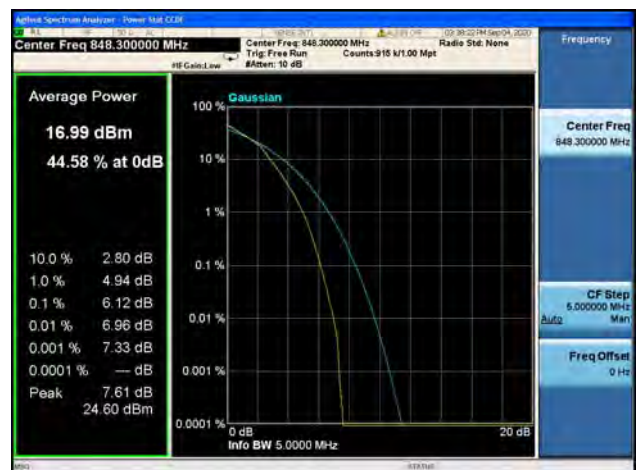
Band5 / 1.4MHz / High CH / 16QAM
