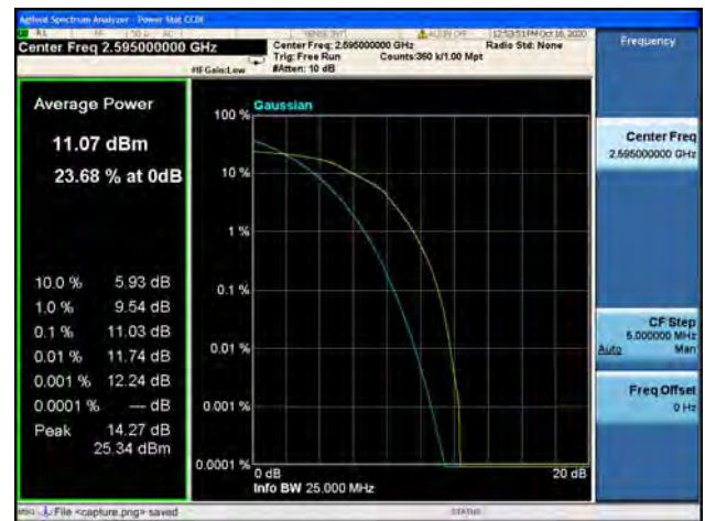
Band38 / 15MHz / High CH / 16QAM
