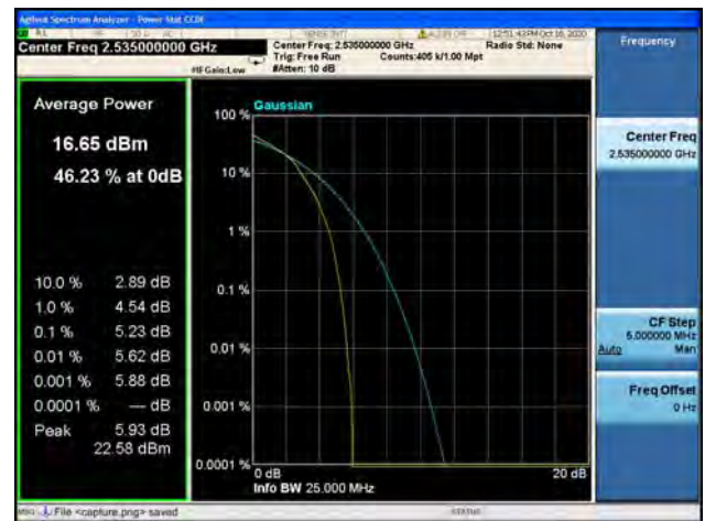
Band7 / 15MHz / High CH / 16QAM
