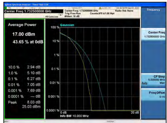
Band4 / 10MHz / High CH / 16QAM
