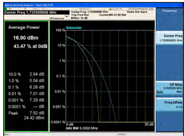
Band4 / 5MHz / High CH / 16QAM
