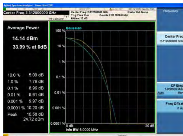
Band40/ Block A / 5MHz / High CH / QPSK
