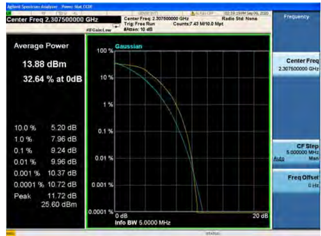
Band40/ Block A / 5MHz / Mid CH / 16QAM
