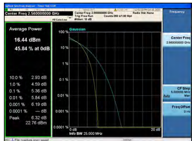
Band7 / 20MHz / High CH / 16QAM
