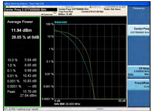
Band38 / 15MHz / Mid CH / 16QAM
