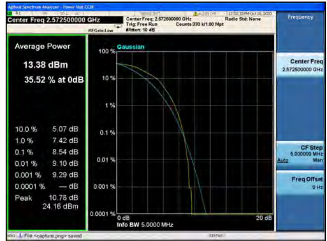
Band38 / 5MHz / Mid CH / 16QAM
