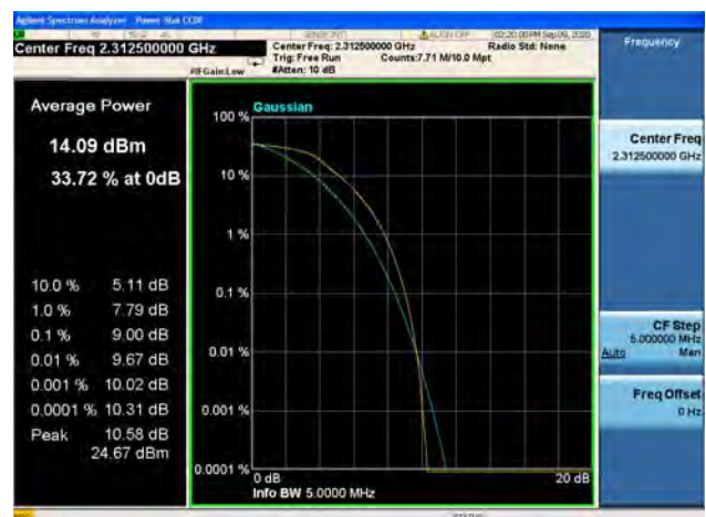
Band40/ Block A / 5MHz / High CH / 16QAM
