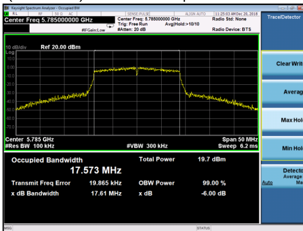
(802.11 n20) 6dB Bandwidth plot on channel 157
