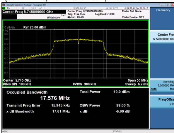
(802.11 n20) 6dB Bandwidth plot on channel 149
