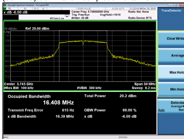
(802.11a) 6dB Bandwidth plot on channel 149
