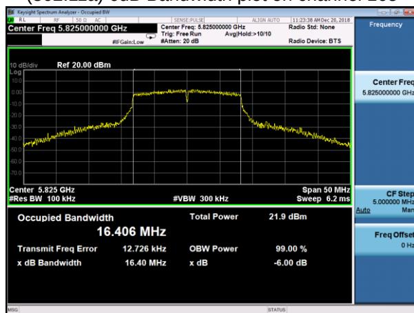
(802.11a) 6dB Bandwidth plot on channel 165
