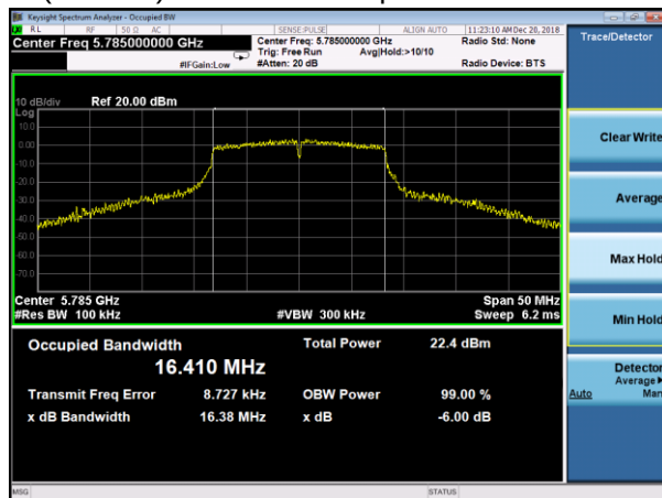
(802.11a) 6dB Bandwidth plot on channel 157
