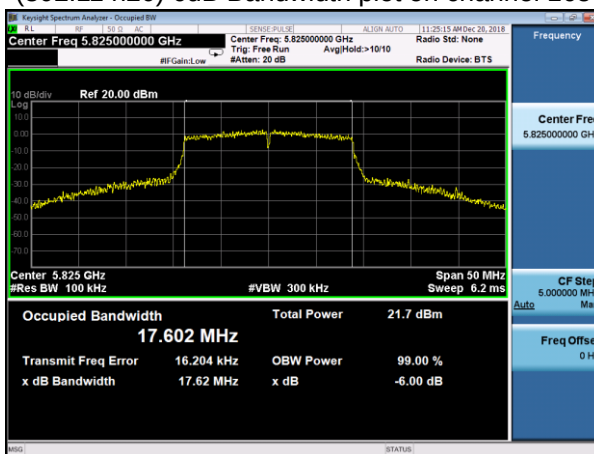
(802.11 n20) 6dB Bandwidth plot on channel 165
