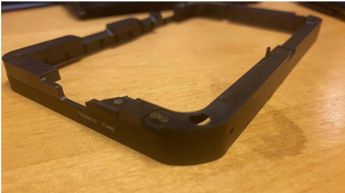
Figur 32 LTE diversity, BT/WiFi and GNSS antenna
