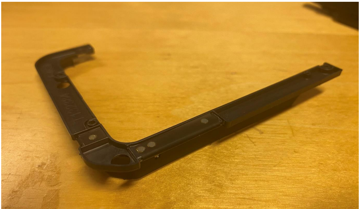
Figur 15 Antenna LTE main, bottom
