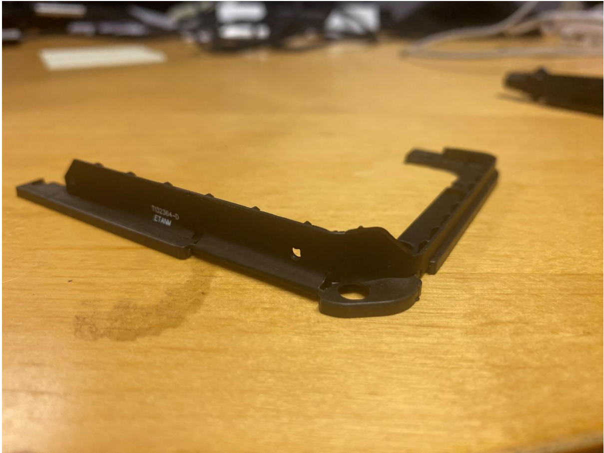
Figur 14 Antenna LTE main
