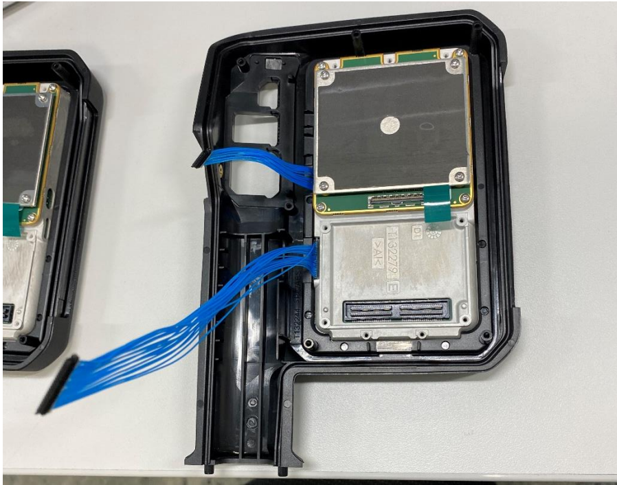
Figur 31 Diversity antenna and cables mounted mounted
