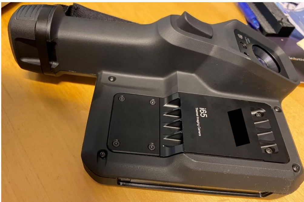
Figur 7 FLIR-i1845 Left side.
