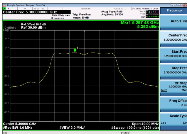
U-NII-2a Power spectral density-802.1 1a(20MHz),5300MHz,Ant1
