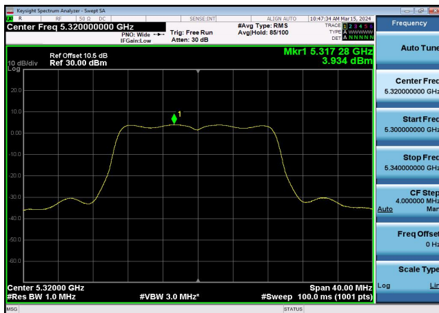
U-NII-2a Power spectral density-802.1 1a(20MHz),5300MHz,Ant1
