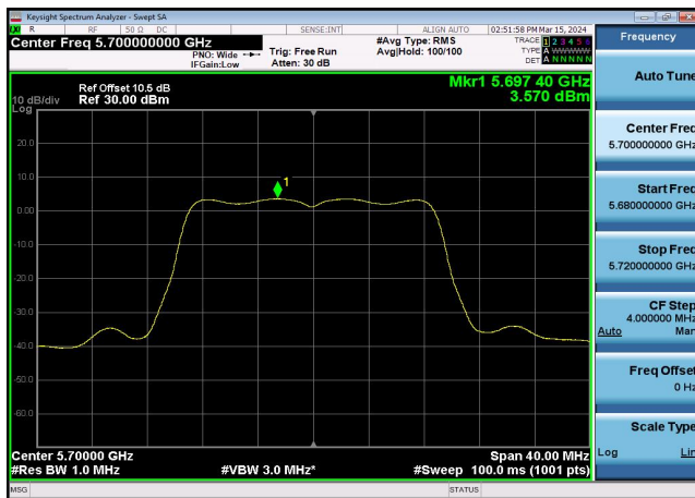
U-NII-2c Power spectral density-802.1 1a(20MHz),5600MHz,Ant1
