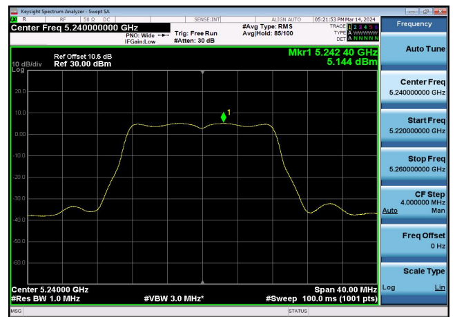
U-NII-1 Power spectral density-802.11 a(20MHz),5240MHz,Ant1
