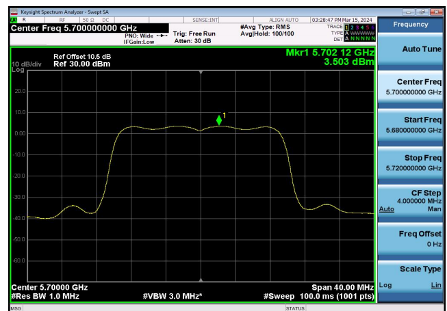
U-NII-2c Power spectral density-802.1 1ax(20MHz),5700MHz,Ant1
