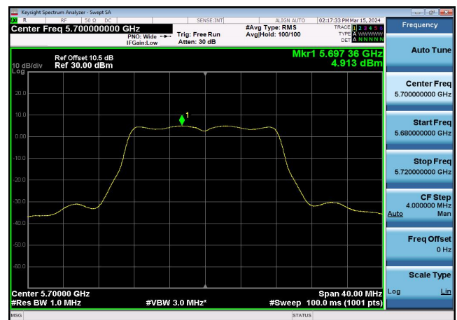
U-NII-2c Power spectral density-802.1 1a(20MHz),5700MHz,Ant1
