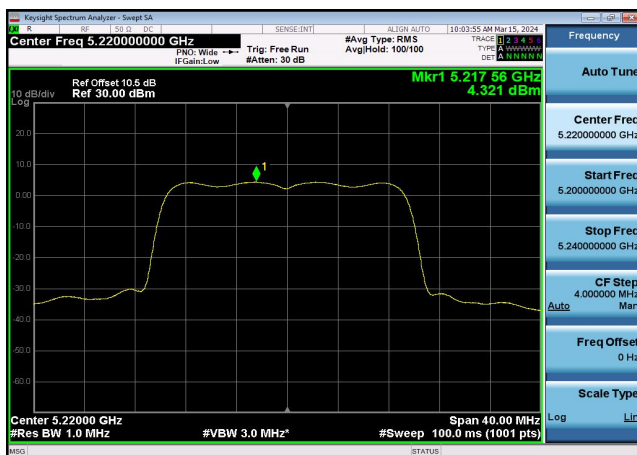
U-NII-1 Power spectral density-802.11 ax(20MHz),5220MHz,Ant1
