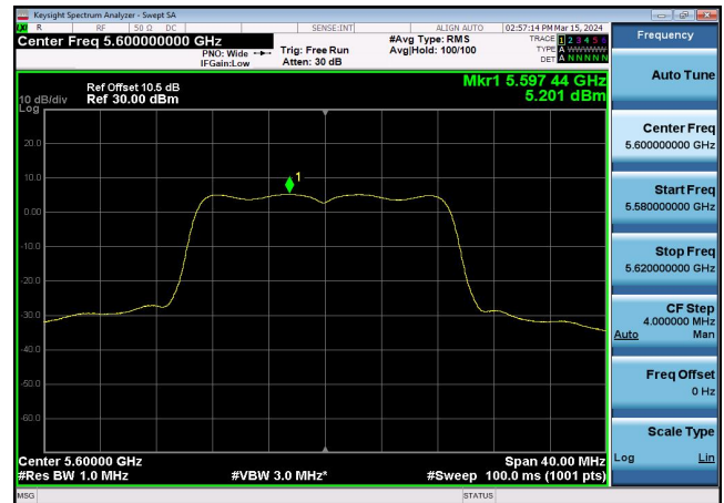
U-NII-2c Power spectral density-802.1 1a(20MHz),5500MHz,Ant1
