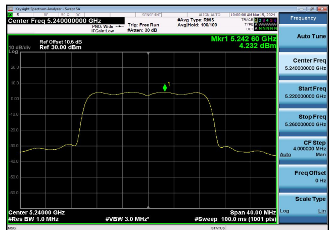
U-NII-1 Power spectral density-802.11 ax(20MHz),5240MHz,Ant1
