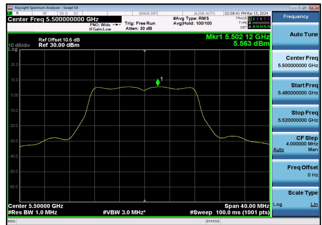
U-NII-2c Power spectral density-802.1 1a(20MHz),5700MHz,Ant1
