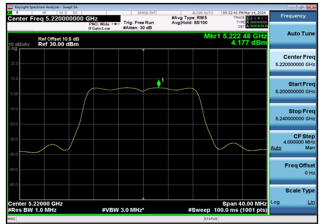
U-NII-1 Power spectral density-802.11 a(20MHz),5180MHz,Ant1
