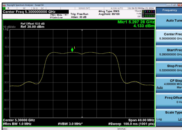
U-NII-2a Power spectral density-802.1 1ax(20MHz),5300MHz,Ant1
