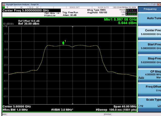
U-NII-2c Power spectral density-802.1 1a(20MHz),5600MHz,Ant1
