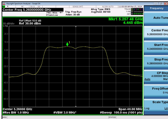
U-NII-2a Power spectral density-802.1 1ac(20MHz),5320MHz,Ant1
