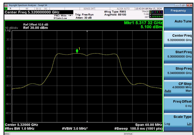
U-NII-2a Power spectral density-802.1 1a(20MHz),5320MHz,Ant1
