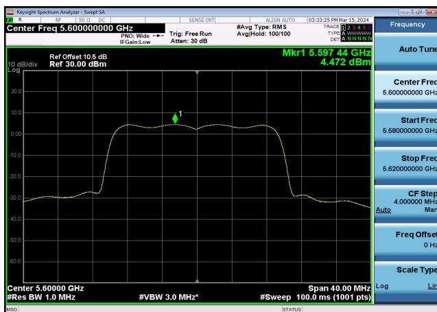
U-NII-2c Power spectral density-802.1 1ax(20MHz),5600MHz,Ant1
