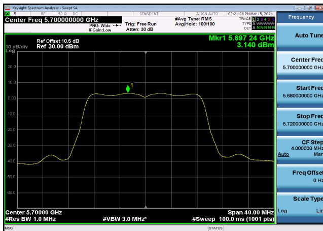
U-NII-2c Power spectral density-802.1 1ax(20MHz),5600MHz,Ant1
