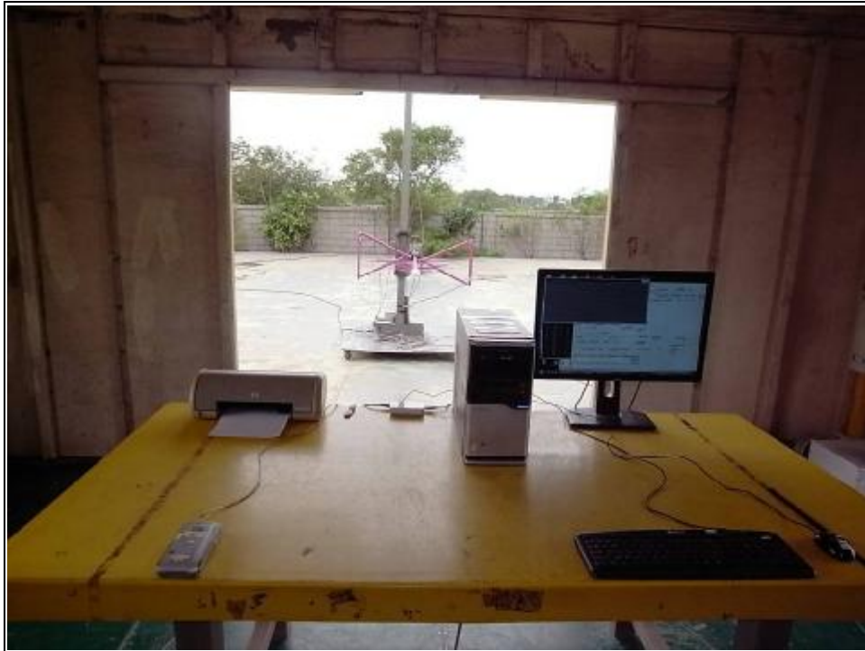
MLWG3 - Radiated test (below 1G , Tx, Standby)
