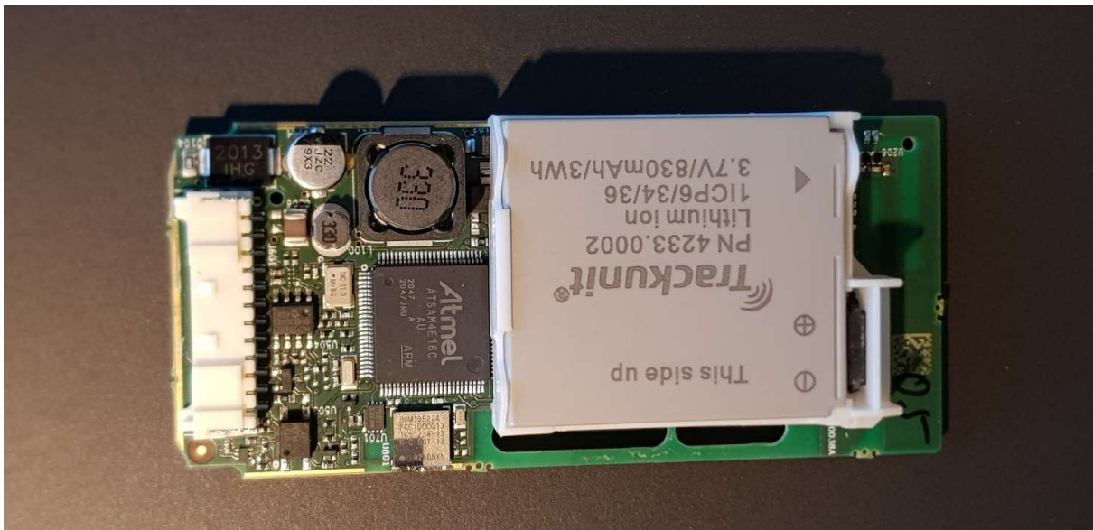
TU600A Print seen from the top with battery model 1-830mAh (Actec)
