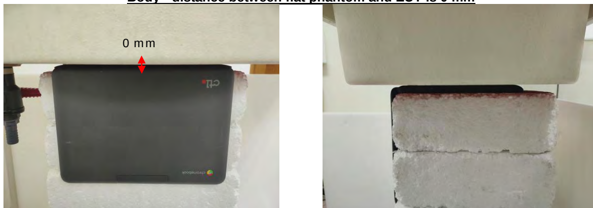
Fig.3 EUT Bottom side to flat phantom
