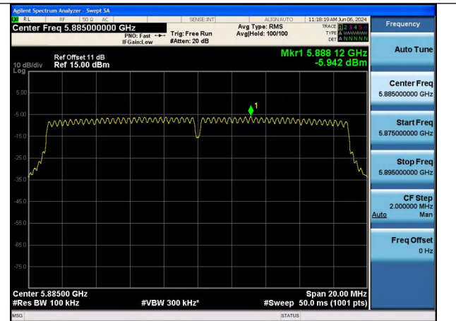
Mode:802.11ac VHT20 Frequency:5885MHz Ant:Chain0
