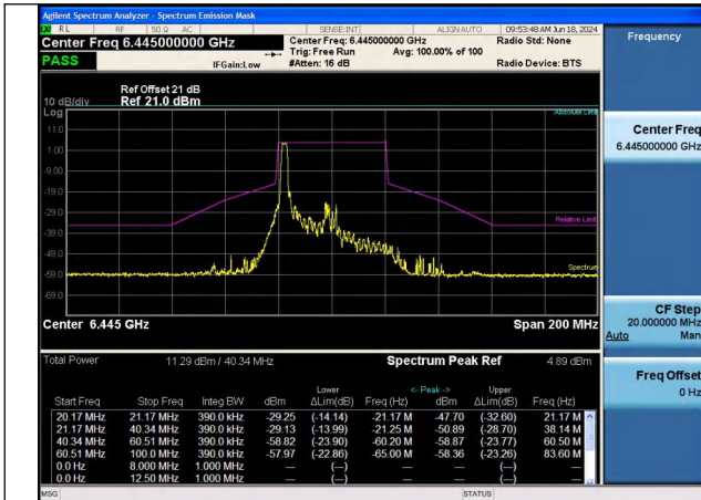
Mode:802.11ax HE40 Tone:26T Frequency:6445MHz Ant:Chain0
