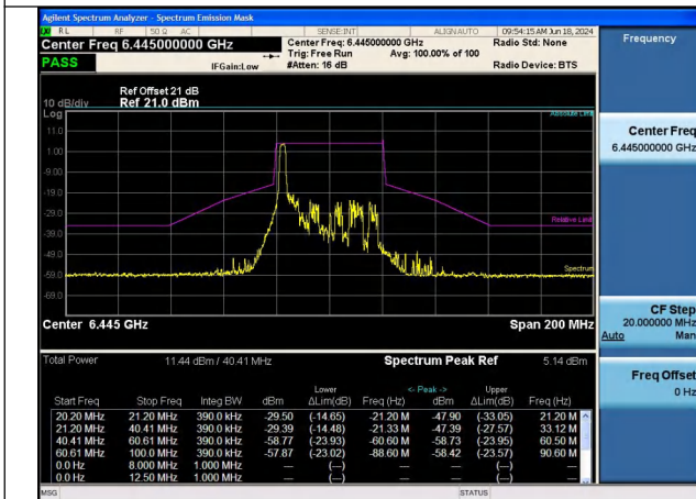
Mode:802.11ax HE40 Tone:26T Frequency:6445MHz Ant:Chain1
