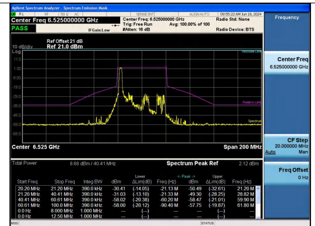
Mode:802.11ax HE40 Tone:26T Frequency:6525MHz Ant:Chain1
