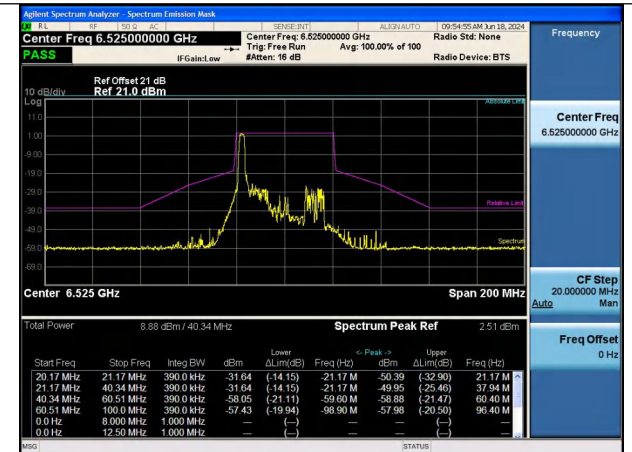
Mode:802.11ax HE40 Tone:26T Frequency:6525MHz Ant:Chain0
