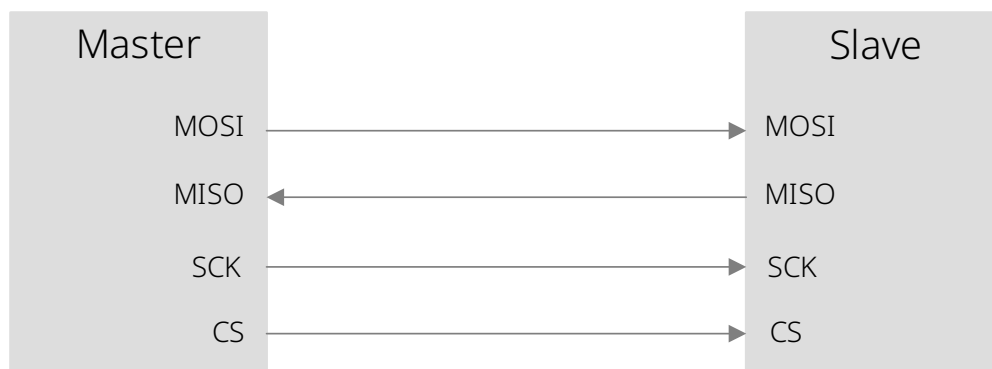
Figure 19. SPI interface reference circuit
