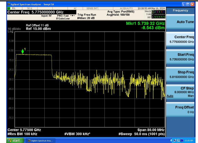
Mode:802.11ax HE80 Tone:242T Frequency:5775MHz Ant:Chain1
