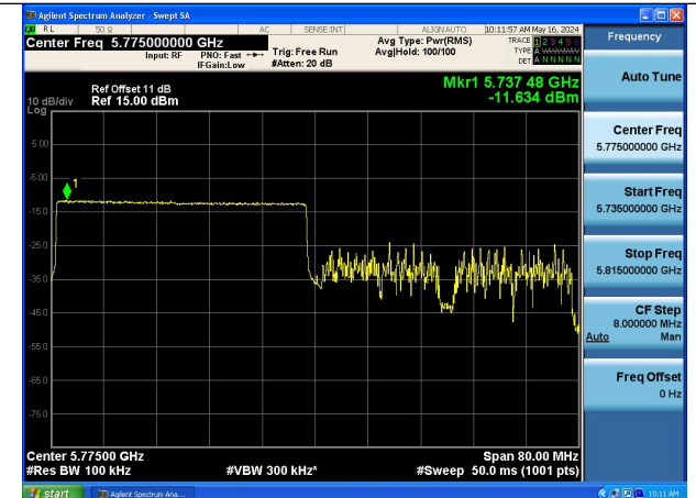
Mode:802.11ax HE80 Tone:484T Frequency:5775MHz Ant:Chain1
