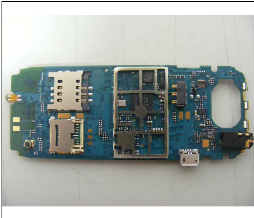
Bottom view of main board (Removing Shield)
