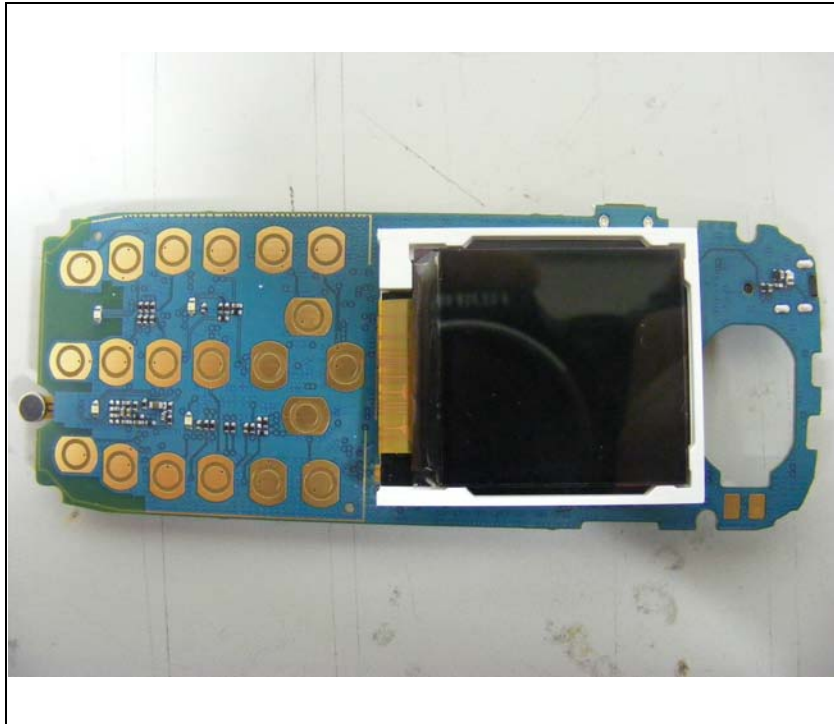
Top view of main board (Bottom of LCD module)
