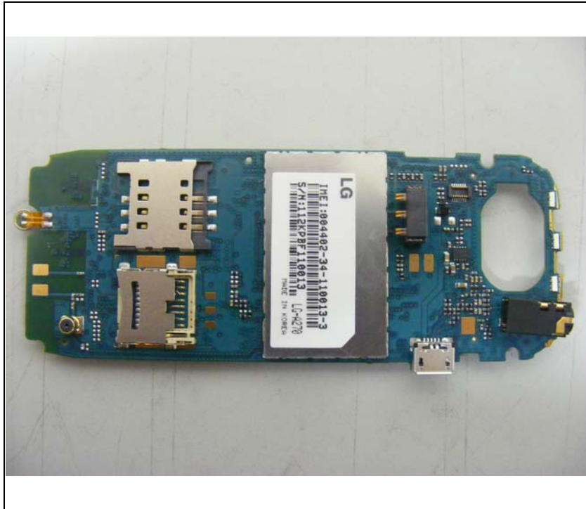
Bottom view of main board (Removing Shield)
