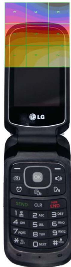
Figure 17-5 H-Field WD Scan overlay
