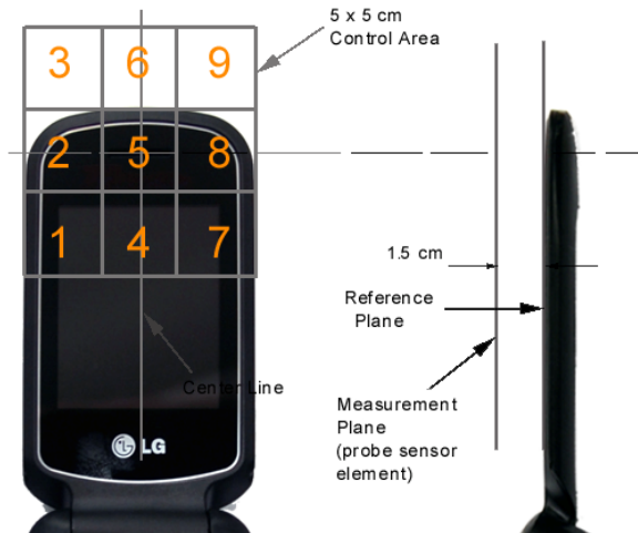
Figure 17-3 5x5 Scan grid above WD
