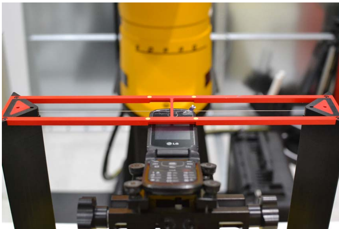
Figure 17-1 Ear Reference Point HAC Phantom Alignment
