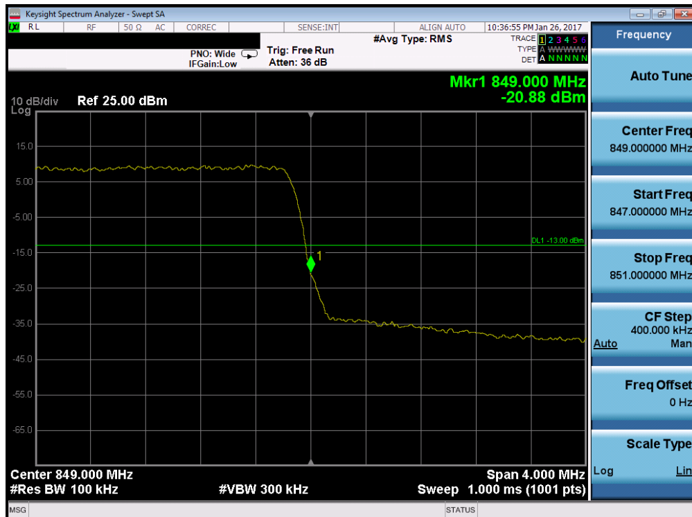
Plot 7-88. Upper Band Edge Plot (Band 5 – 3.0MHz QPSK – RB Size 15)
