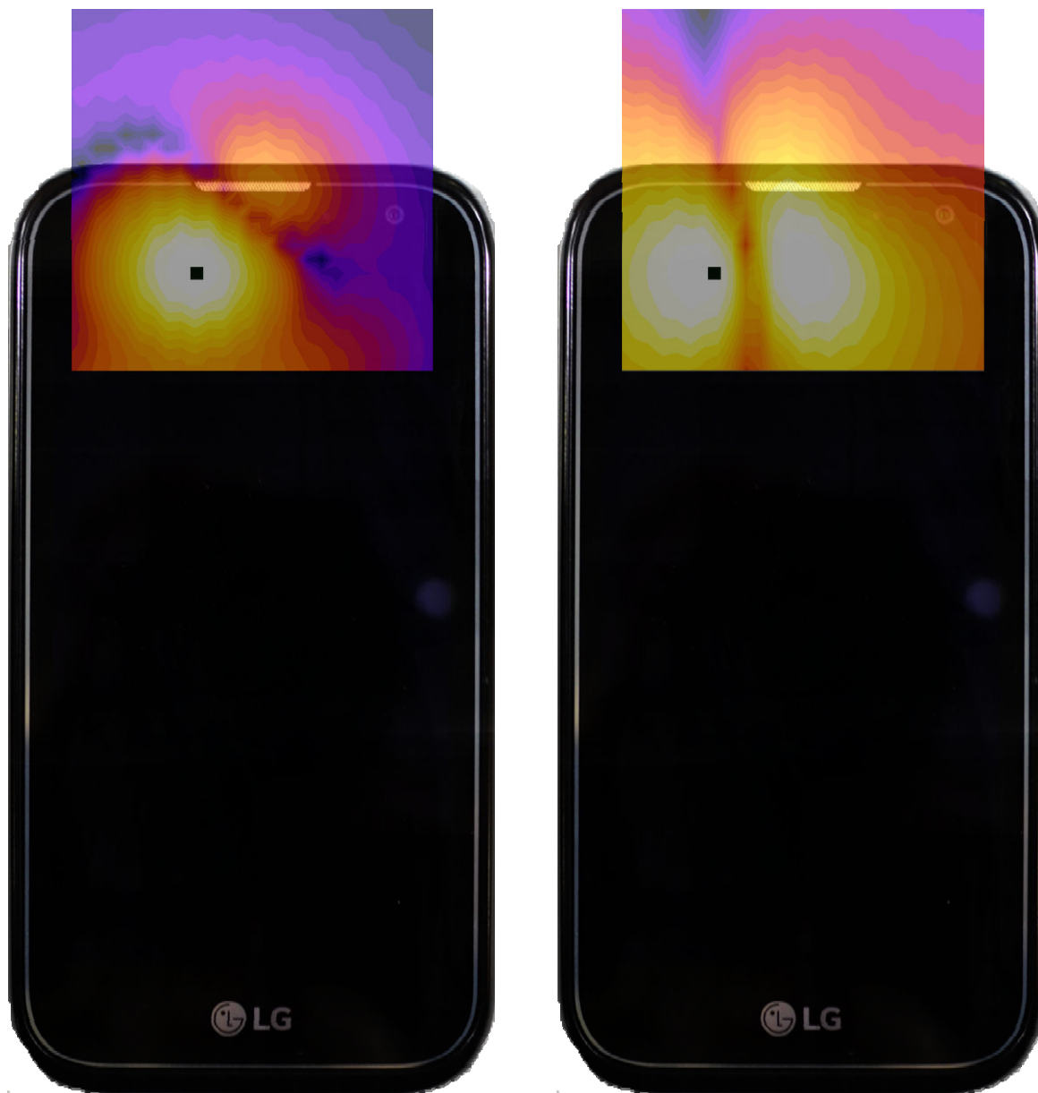
Figure 13-3 T-Coil Scan Overlay Magnetic Field Distributions
