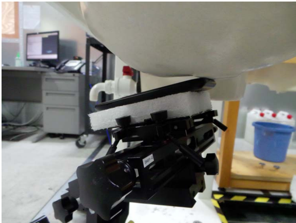
SAR Test Setup Photo 4: Left Tilt
