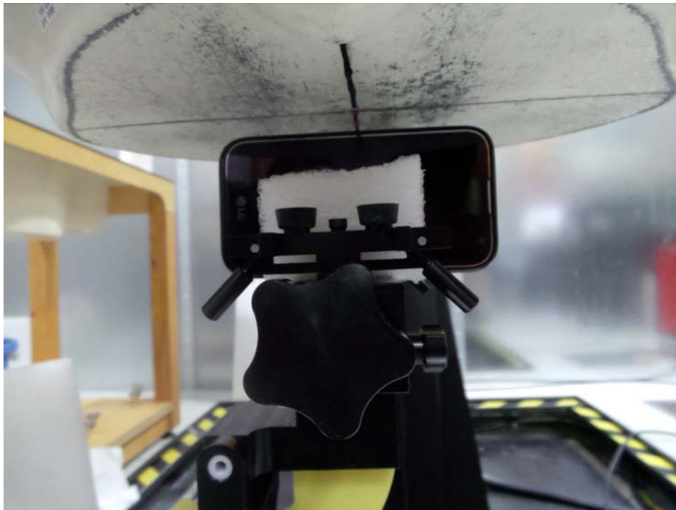
SAR Test Setup Photo 10: Left Edge at 10 mm
