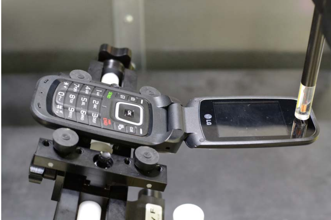
Figure 13-1 Test Setup for Wireless Device
