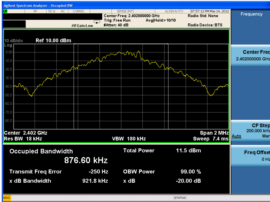
Plot 6-1. 20dB Bandwidth Plot (Bluetooth, 1Mbps – Ch. 0)
