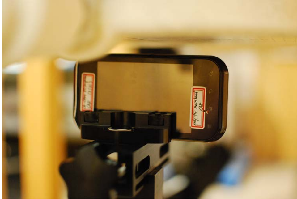
SAR Test Setup Photo 9: Right at 1.0 cm
