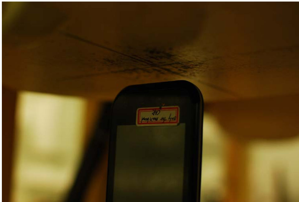
SAR Test Setup Photo 8: Bottom at 1.0 cm
