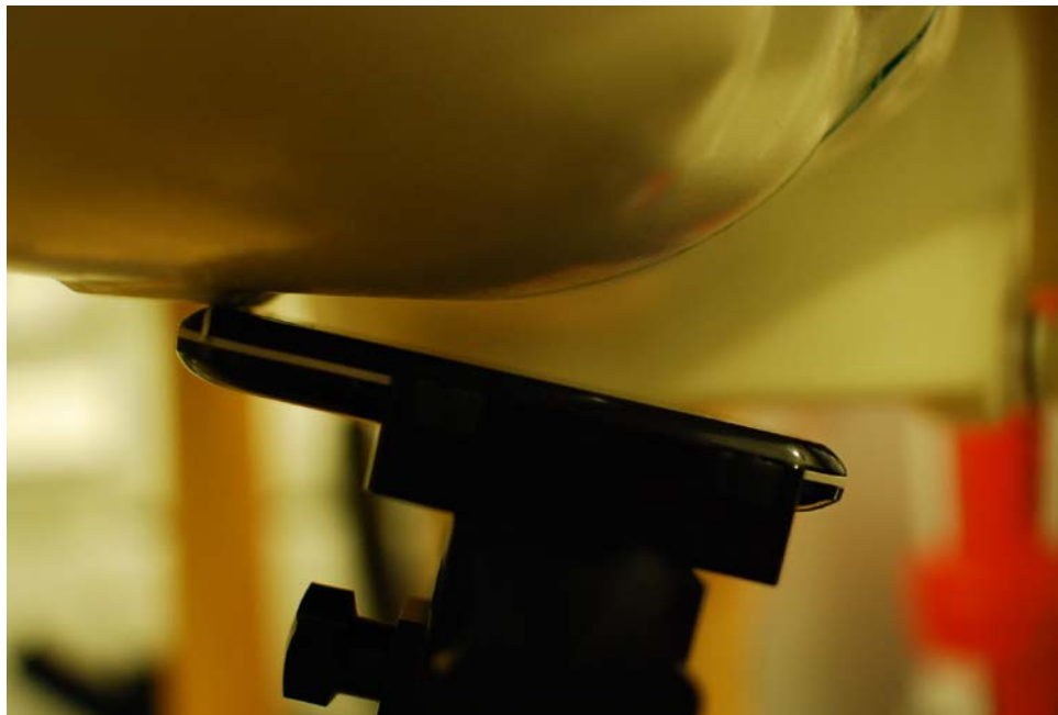
SAR Test Setup Photo 2: Right Tilt
