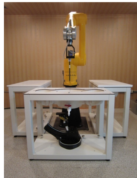
Figure 2.2 DASY5 Test System
