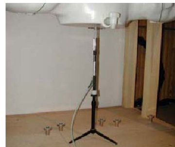
Figure 11.1 Dipole Verification Test Setup Diagram & Photo
