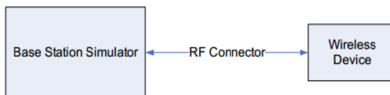
Figure 10.2 Power Measurement Setup
