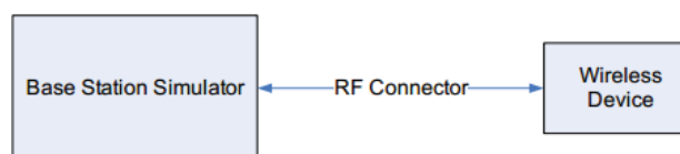
Figure 10.1 Power Measurement Setup
