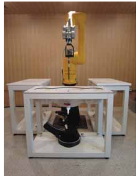
Figure 2.2 DASY5 Test System
