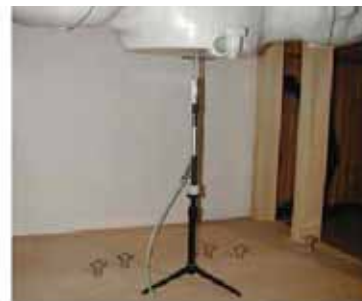
Figure 11.1 Dipole Verification Test Setup Diagram & Photo
