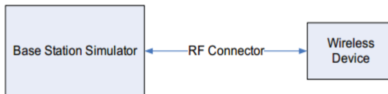
Figure 10.2 Power Measurement Setup
