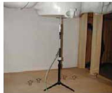
Figure 11.1 Dipole Verification Test Setup Diagram & Photo
