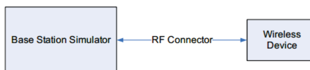
Figure 10.1 Power Measurement Setup
