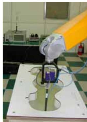
Figure 5. Photograph of the probe and the Phantom
