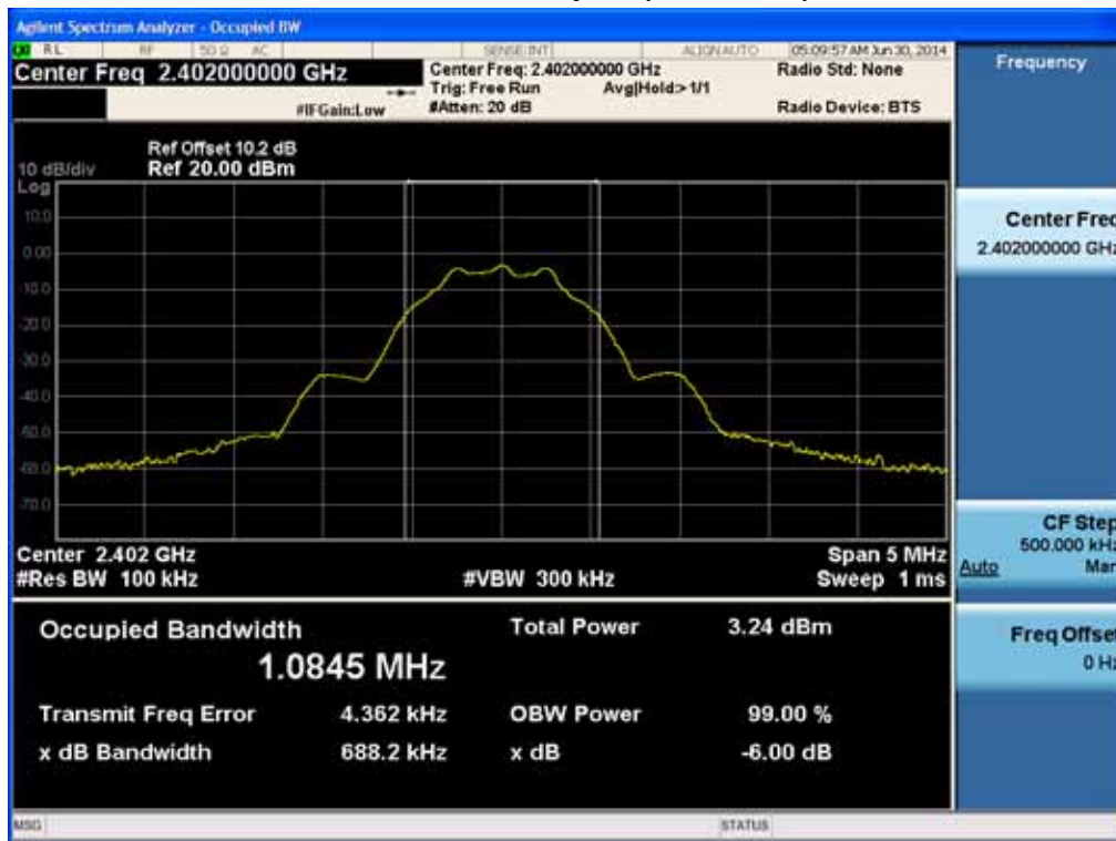
6dB Bandwidth plot (Low-CH 0)
