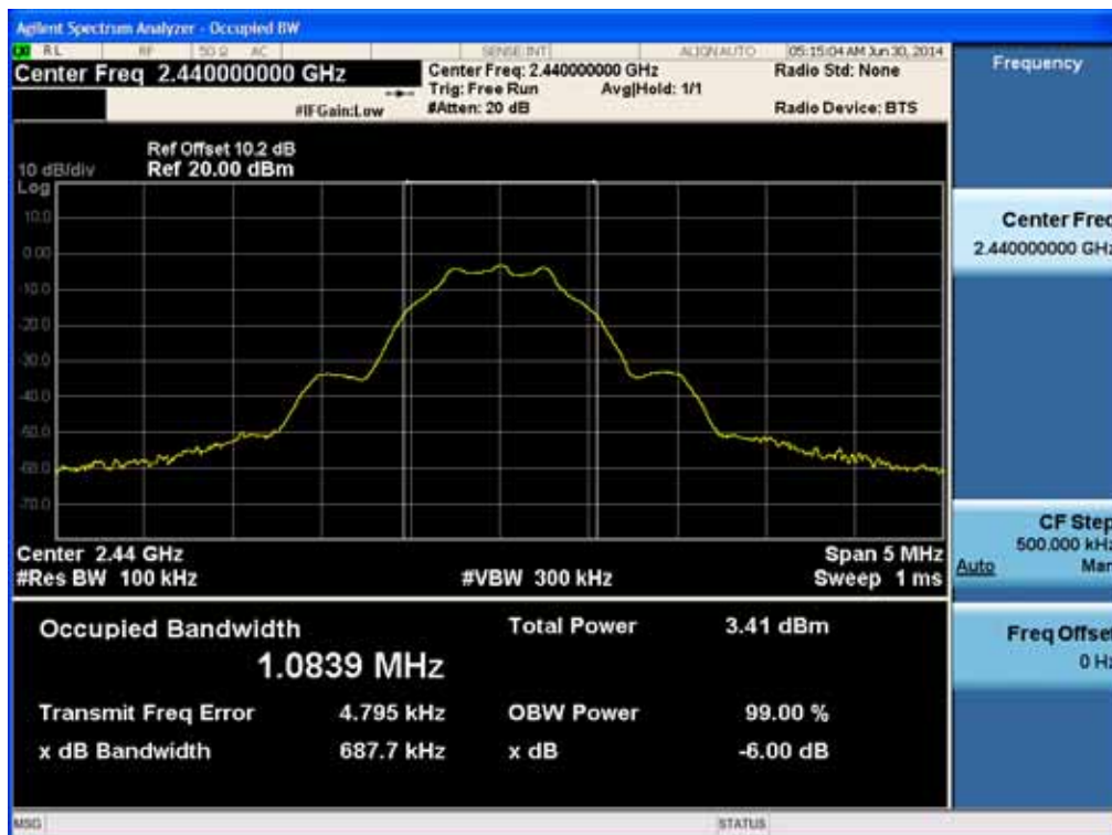
6dB Bandwidth plot (Mid-CH 19)
