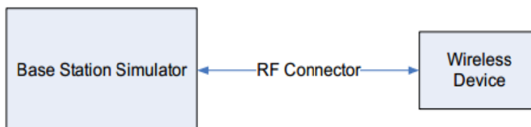
Figure 10.2 Power Measurement Setup
