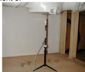
Figure 11.1 Dipole Verification Test Setup
