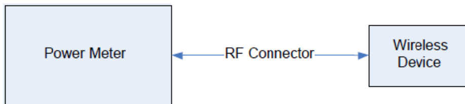
Figure 10.4 Power Measurement Setup
