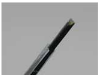
Figure 6. EX3DV4 E-field Probe
