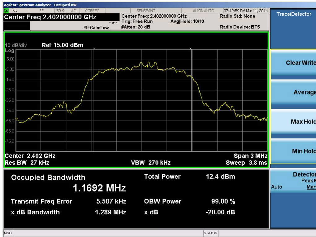
Plot 6-7. 20dB Bandwidth Plot (Bluetooth, 3Mbps – Ch. 0)
