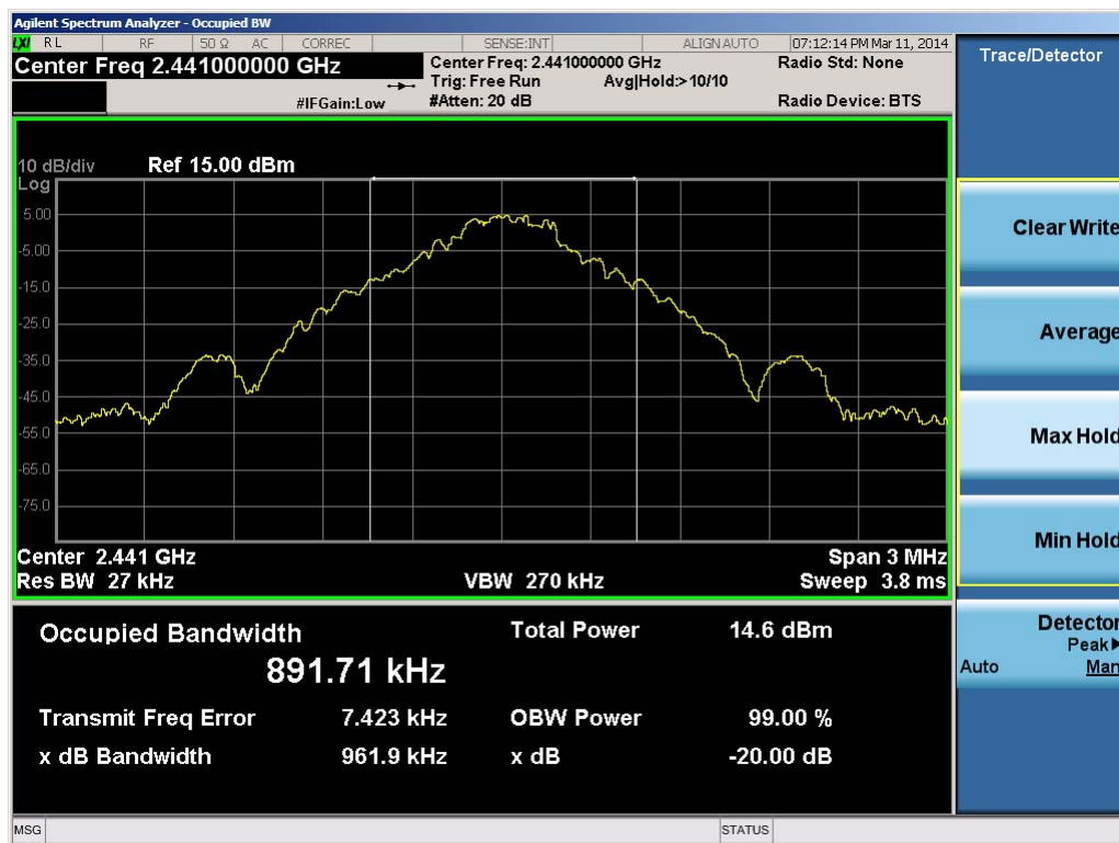
Plot 6-2. 20dB Bandwidth Plot (Bluetooth, 1Mbps – Ch. 39)
