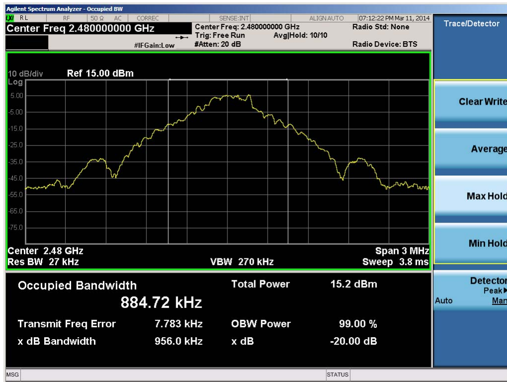
Plot 6-3. 20dB Bandwidth Plot (Bluetooth, 1Mbps – Ch. 78)
