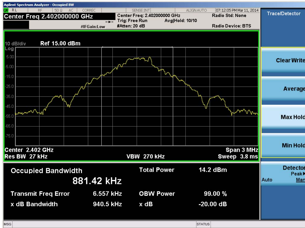
Plot 6-1. 20dB Bandwidth Plot (Bluetooth, 1Mbps – Ch. 0)
