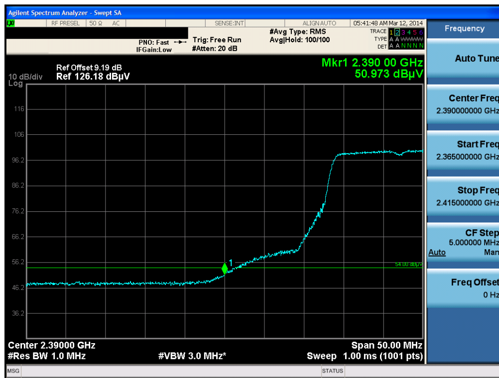
Plot 6-31. Radiated Restricted Lower Band Edge Measurement (Average)
