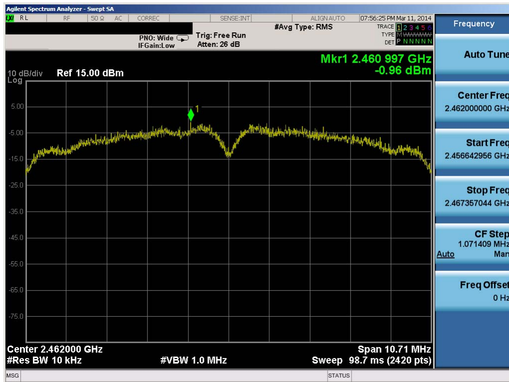
Plot 6-12. Power Spectral Density Plot (802.11b – Ch. 11)
