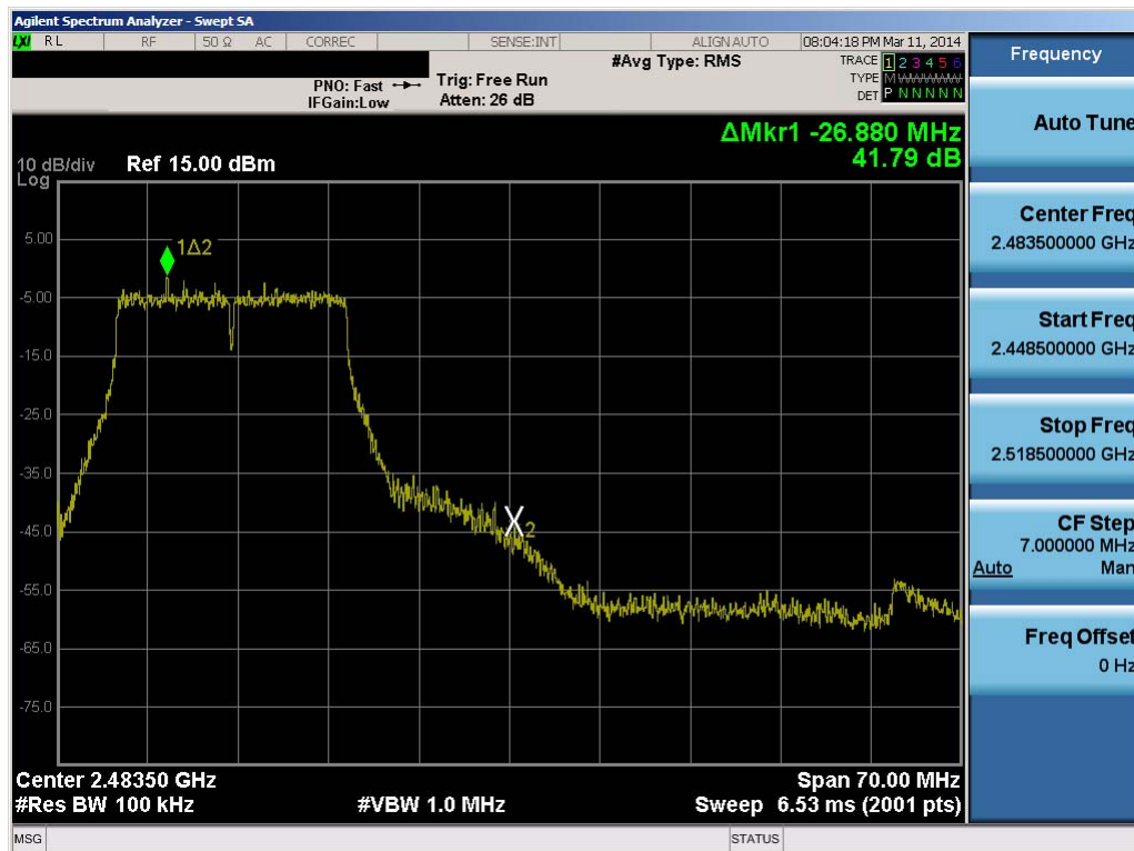
Plot 6-24. Band Edge Plot (802.11n (2.4GHz) – Ch. 11)
