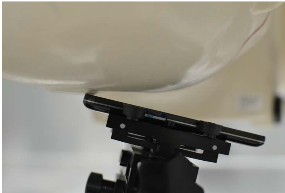
SAR Test Setup Photo 2 – Right Tilt
