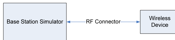
Figure 9-1 Power Measurement Setup
