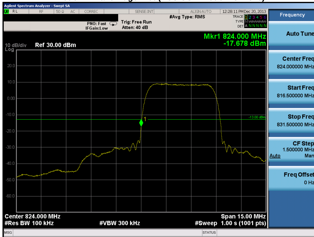
Plot 6-45. Band Edge Plot (Cellular WCDMA Mode – Ch. 4132)
