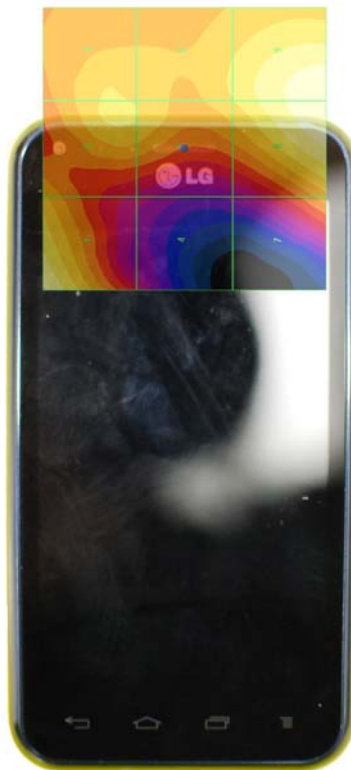
Figure 18-4 E-Field WD Scan overlay
