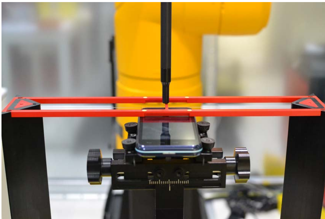
Figure 18-1 Ear Reference Point HAC Phantom Alignment
