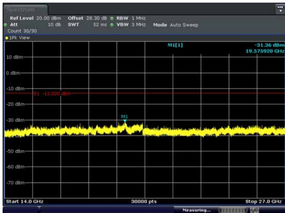
Conducted Spurious Plot 2 (15MHz Ch.21100 QPSK RF 1, Offset 0)
