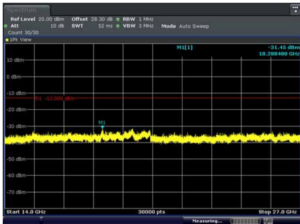
Conducted Spurious Plot 2 (20MHz Ch.21100 QPSK RF 1, Offset 0)
