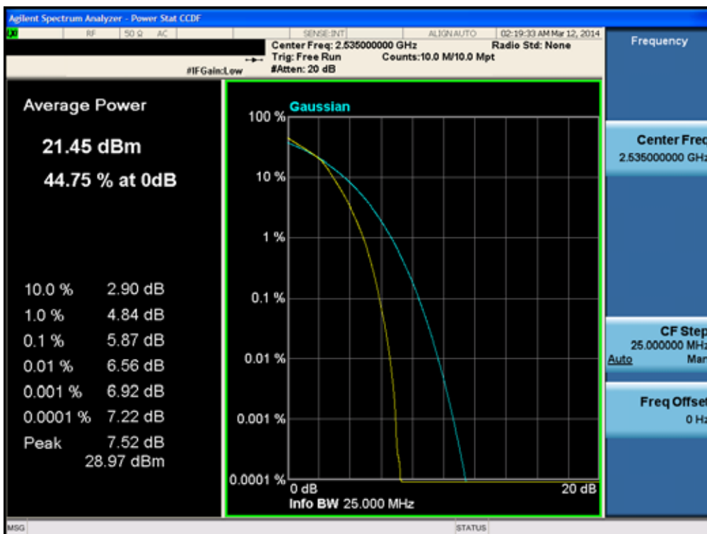
Peak to Average Ratio Plot (15MHz Ch.21100 16-QAM RB 75)
