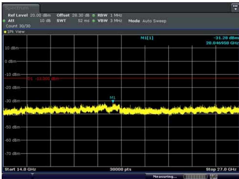
Conducted Spurious Plot 2 (15MHz Ch.21375 QPSK RF 1, Offset 0)
