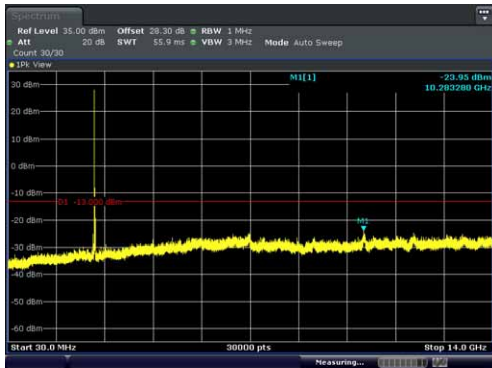
Conducted Spurious Plot 1 (20MHz Ch.21100 QPSK RF 1, Offset 0)
