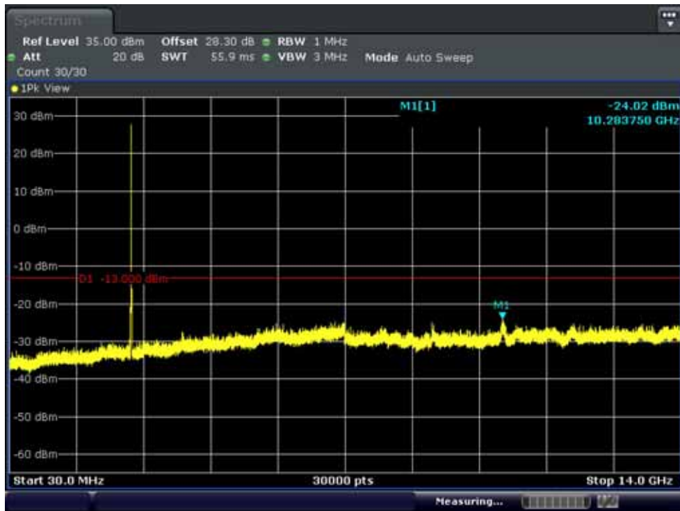
Conducted Spurious Plot 1 (15MHz Ch.21375 QPSK RF 1, Offset 0)
