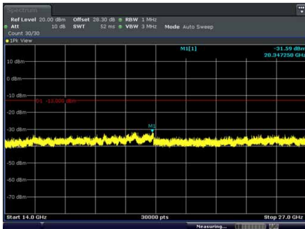
Conducted Spurious Plot 2 (10MHz Ch.21400 QPSK RF 1, Offset 0)
