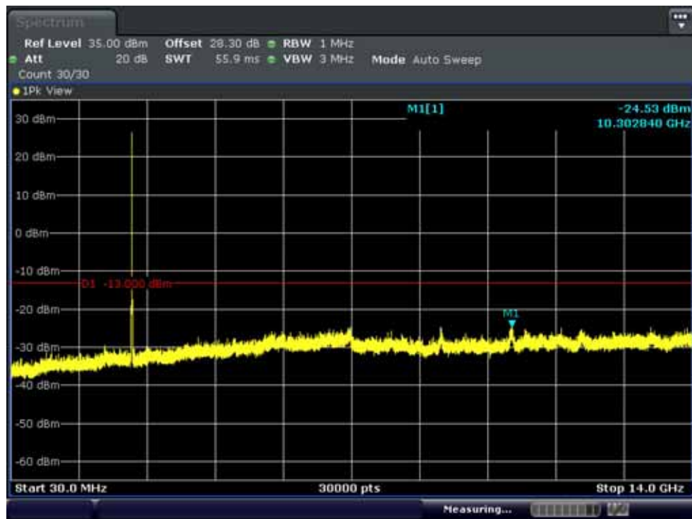
Conducted Spurious Plot 1 (15MHz Ch.20825 QPSK RF 1, Offset 0)
