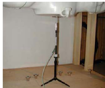
Figure 11.1 Dipole Verification Test Setup Diagram & Photo
