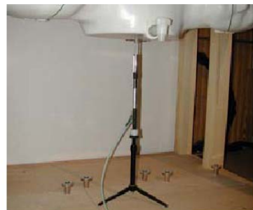
Figure 11.1 Dipole Verification Test Setup Diagram & Photo
