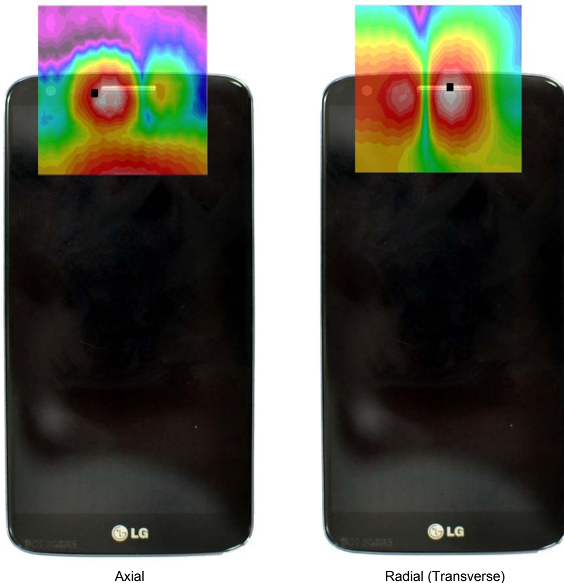
Figure 13-3 T-Coil Scan Overlay Magnetic Field Distributions
