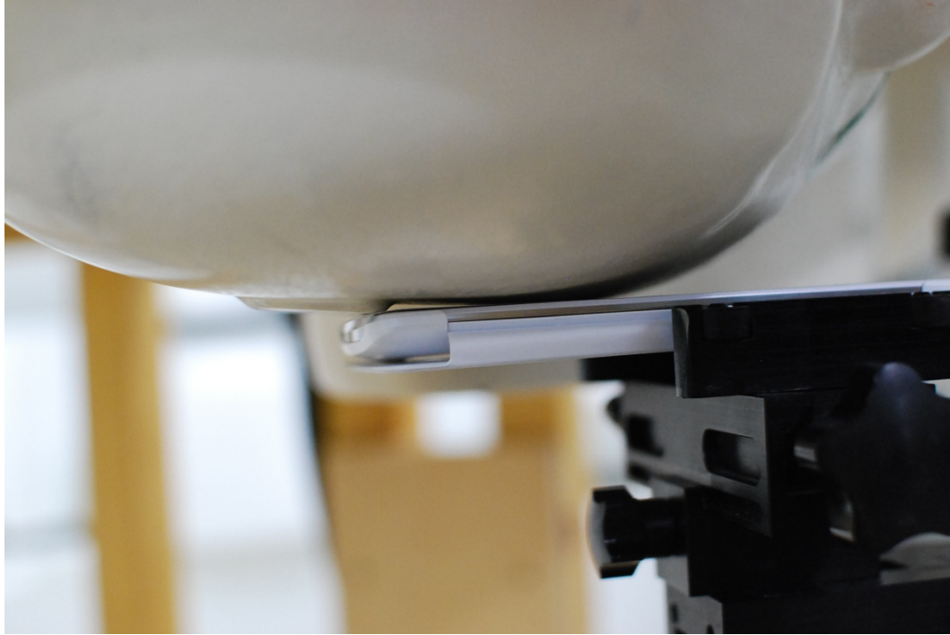
SAR Test Setup Photo 3 - Right Cheek with WCC open
