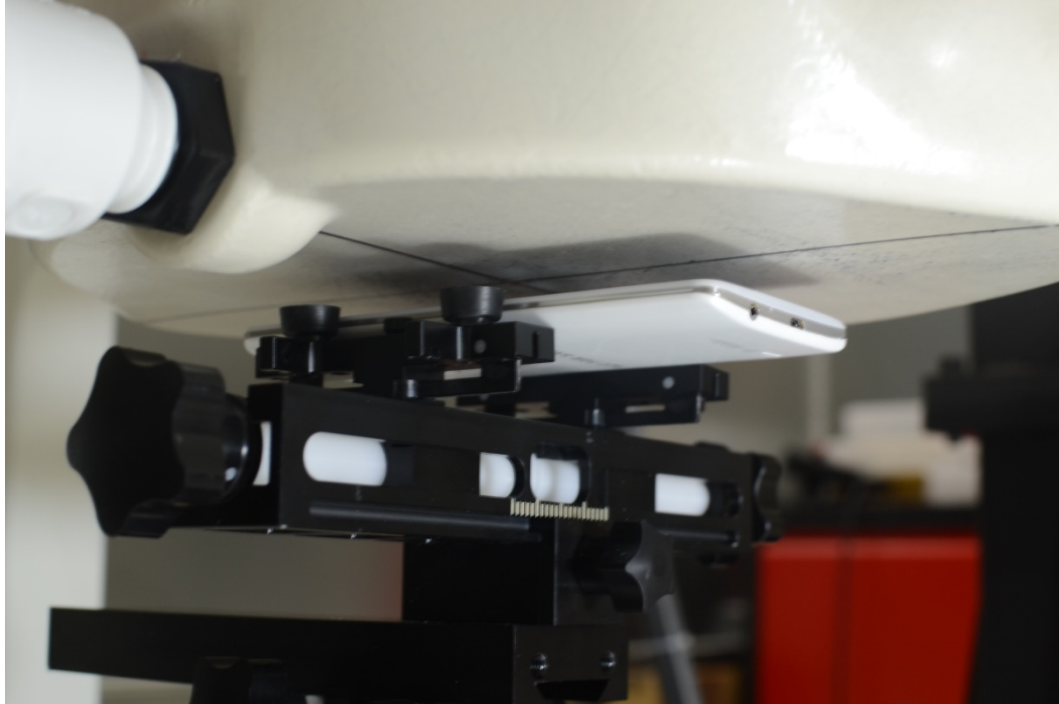
SAR Test Setup Photo 13 - Front at 10 mm
