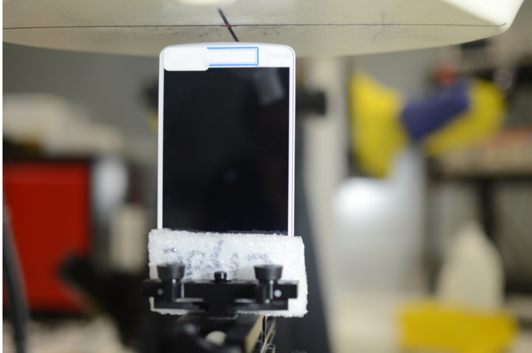
SAR Test Setup Photo 15 - Bottom at 10 mm
