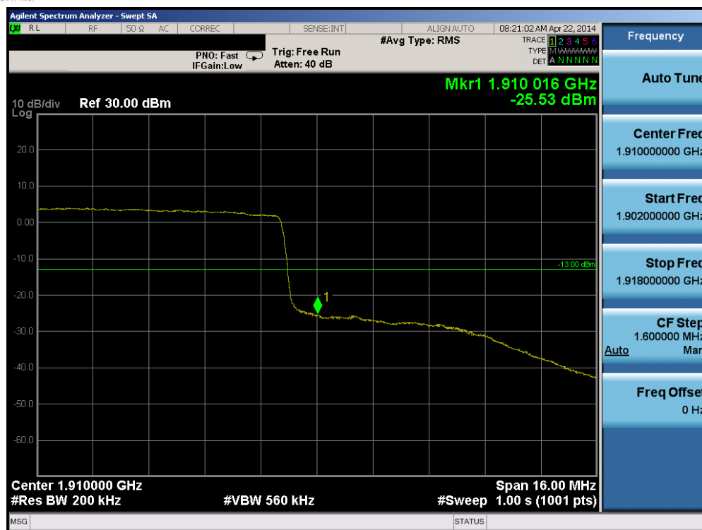
Plot 6-133. Upper Band Edge Plot (Band 2 – 20.0MHz QPSK – RB Size 100)
