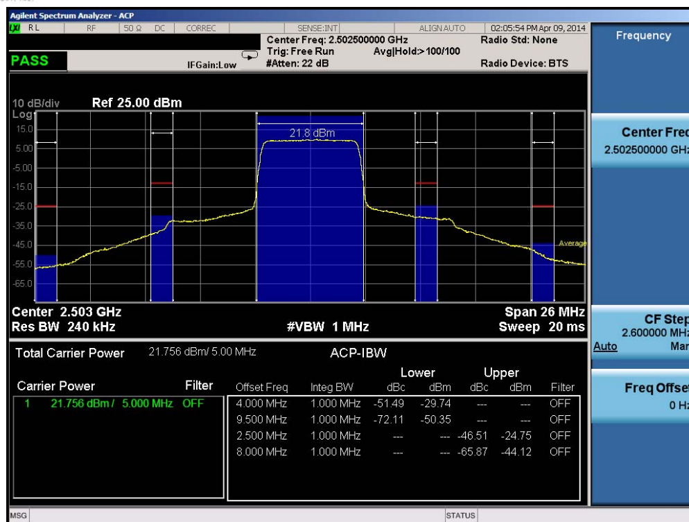
Plot 6-137. Lower ACP Plot (Band 7 – 5.0MHz QPSK – RB Size 25)
