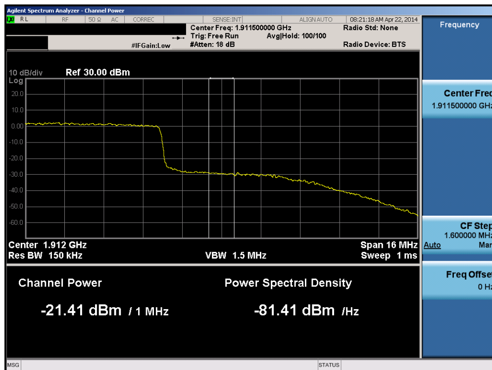
Plot 6-134. Upper Extended Band Edge Plot (Band 2 – 20.0MHz QPSK – RB Size 100)
