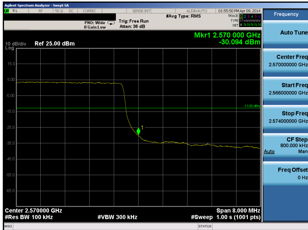
Plot 6-142. Upper Band Edge Plot (Band 7 – 10.0MHz QPSK – RB Size 50)
