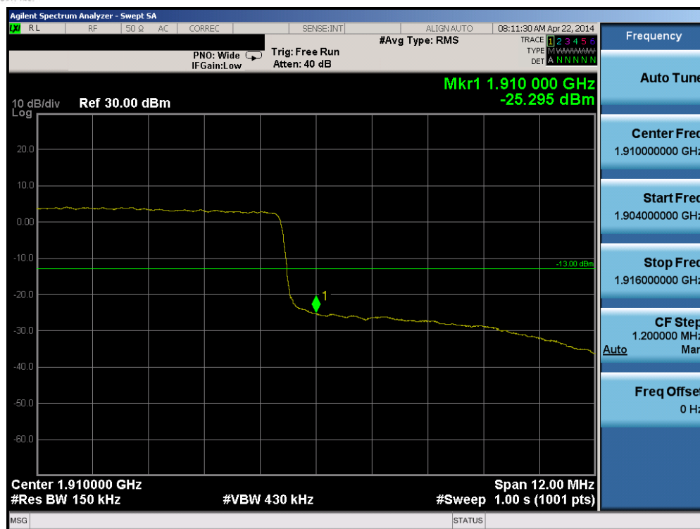
Plot 6-129. Upper Band Edge Plot (Band 2 – 15.0MHz QPSK – RB Size 75)
