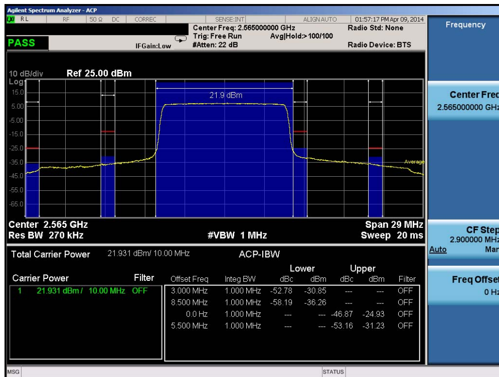
Plot 6-146. Upper ACP Plot (Band 7 – 10.0MHz QPSK – RB Size 50)
