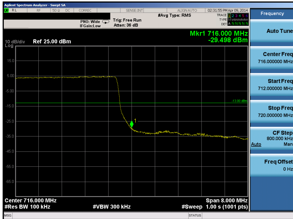
Plot 6-102. Upper Band Edge Plot (Band 17 – 10.0MHz QPSK – RB Size 50)
