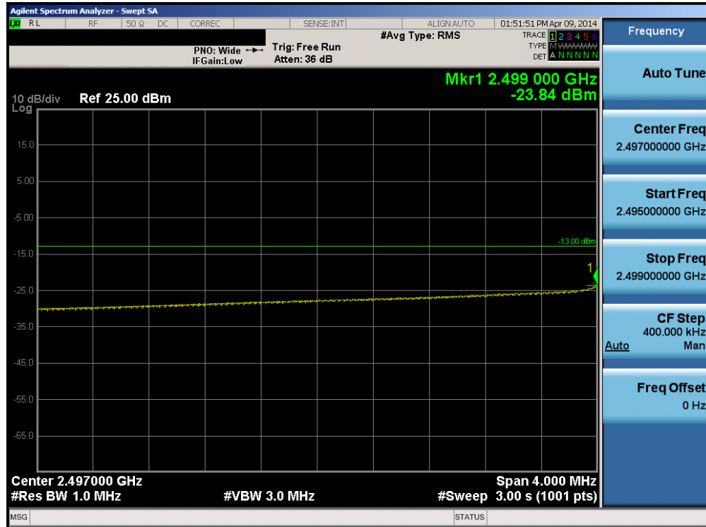
Plot 6-141. Lower Extended Band Edge Plot (Band 7 – 10.0MHz QPSK – RB Size 50)
