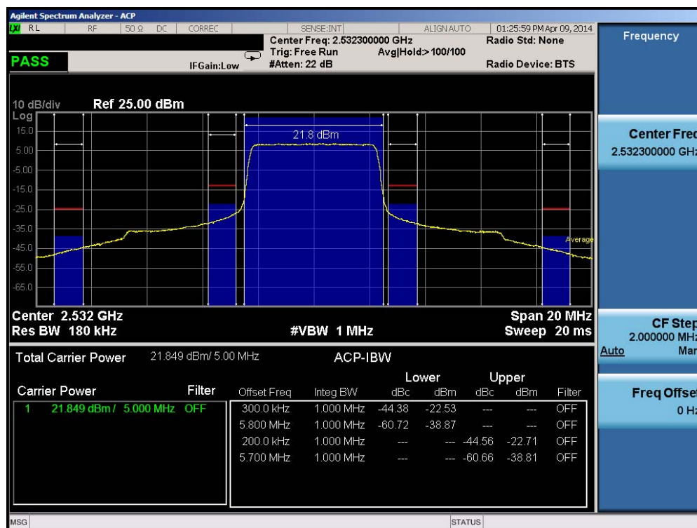
Plot 6-138. Mid ACP Plot (Band 7 – 5.0MHz QPSK – RB Size 25)
