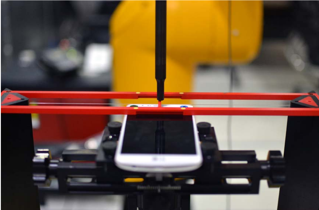
Figure 18-1 Ear Reference Point HAC Phantom Alignment, Standard Battery Cover
