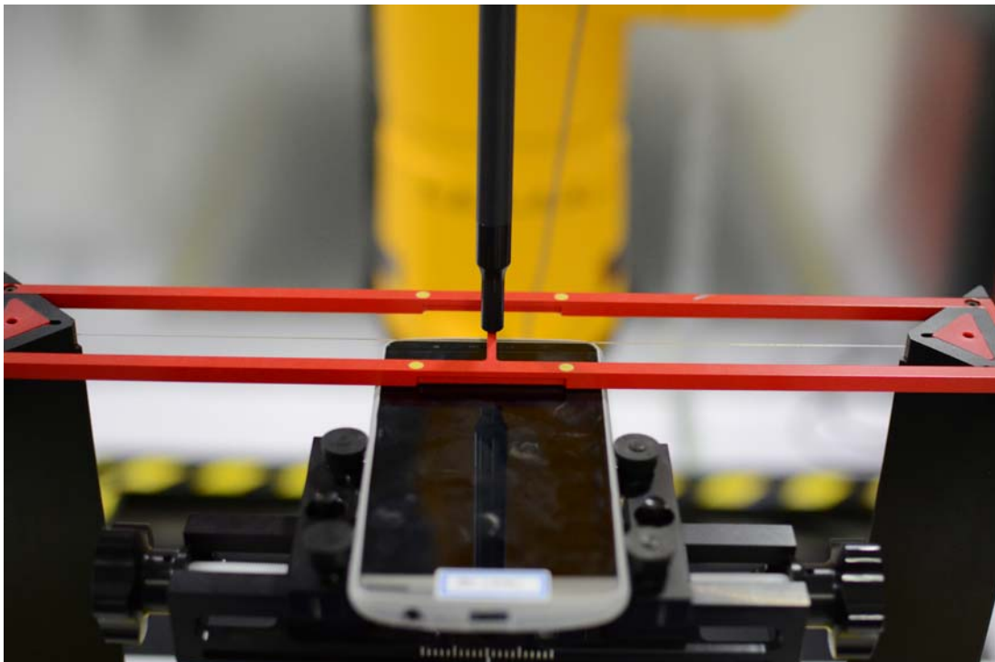
Figure 18-4 Ear Reference Point HAC Phantom Alignment (Wireless Charging Cover)
