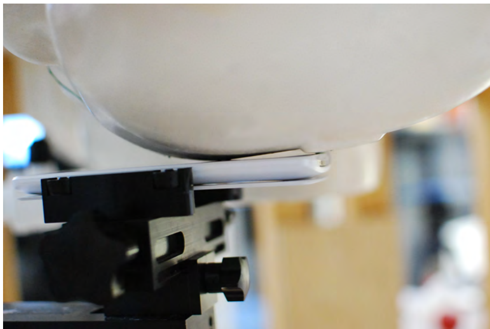
SAR Test Setup Photo 7 – Left Cheek, Wireless Charging Cover, Case Open
