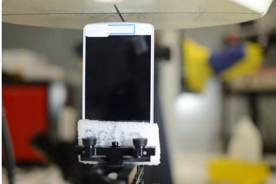
SAR Test Setup Photo 16 – Bottom Edge, Standard Cover at 1.0 cm
