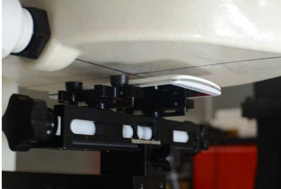
SAR Test Setup Photo 12 – Back Side, Standard Cover at 1.0 cm
