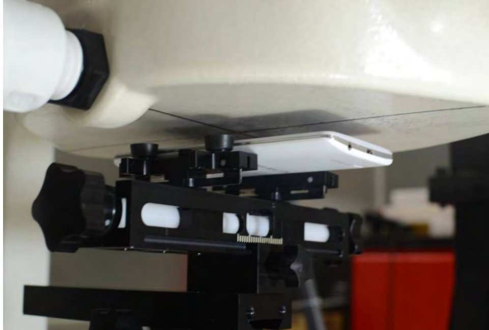
SAR Test Setup Photo 14 – Front Side, Standard Cover at 1.0 cm
