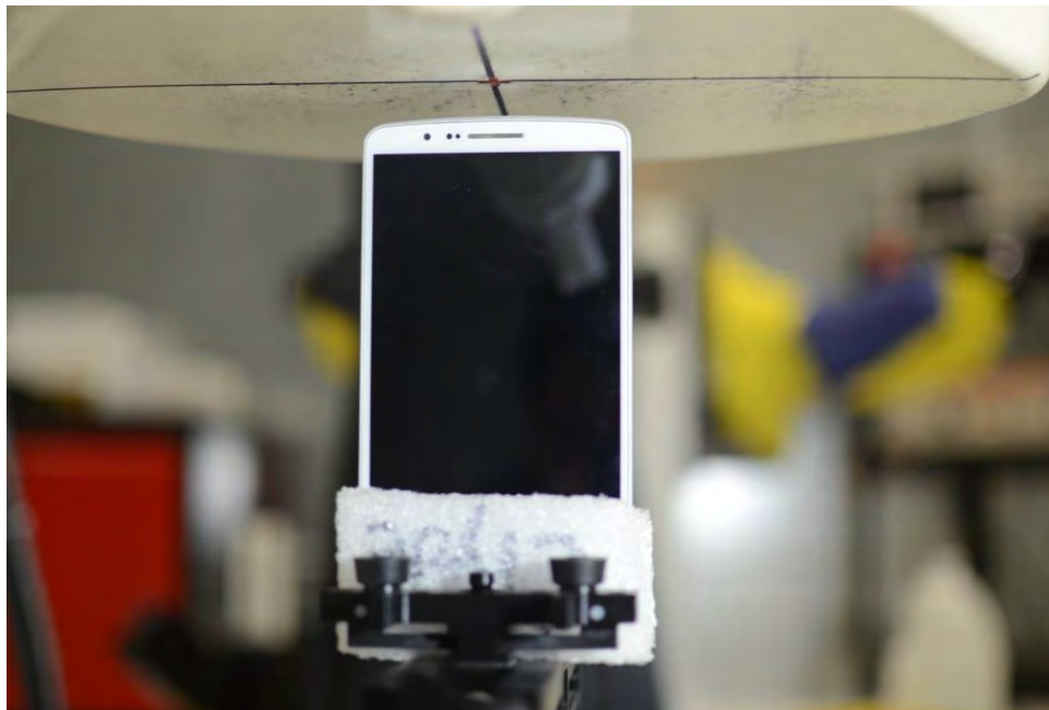
SAR Test Setup Photo 15 – Top Edge, Standard Cover at 1.0 cm
