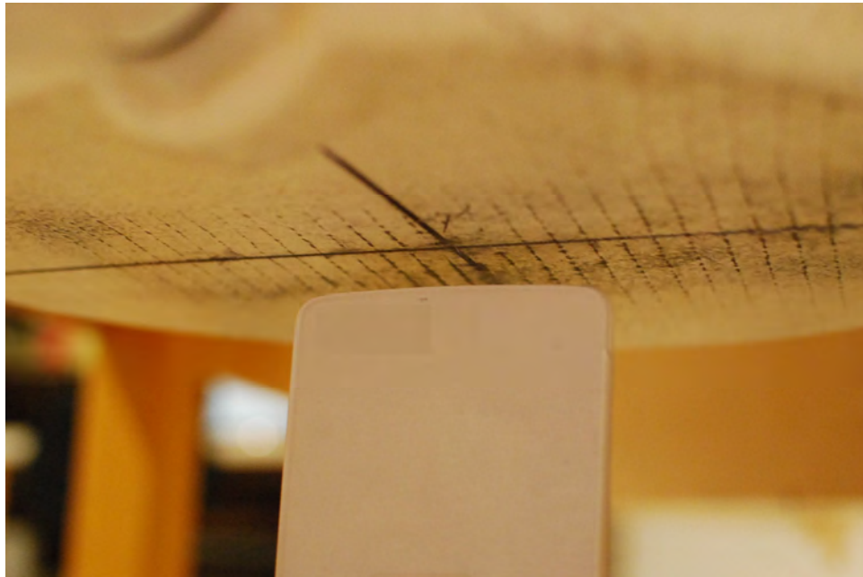
SAR Test Setup Photo 17 – Bottom Edge, Wireless Charging Cover Closed at 1.0 cm
