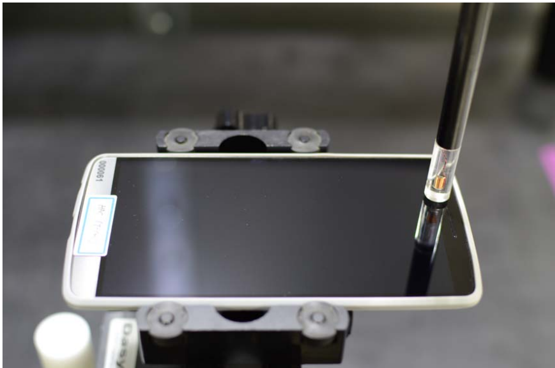
Figure 13-2 Test Setup for Wireless Device (Wireless Charging Cover)
